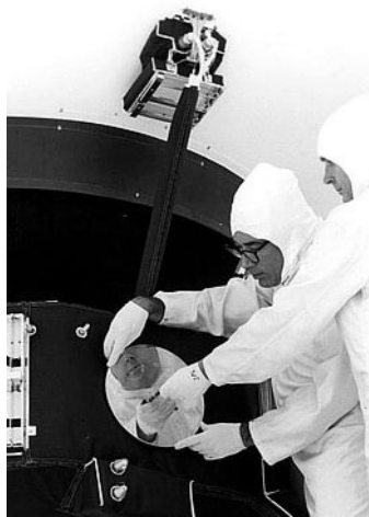
Fig. 3.8. The backs of Voyager 's sun sensors are visible on the white HGA above the heads of the people affixing the famous golden record. Two of the four yaw thrusters can be seen below the record. Image courtesy NASA/JPL.
