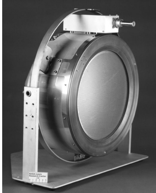
Fig. 4.10. An ion engine capable of 0.09 N thrust, three of which the Dawn spacecraft carries in the main asteroid belt. The high-speed ion exhaust issues from the circular grid, while electrons are expelled from the gun atop the engine. Image courtesy NASA/LRC.
