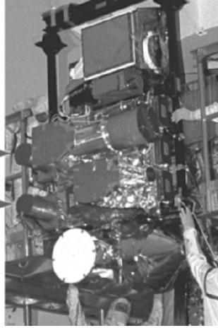
Fig. B.11. Two SRUs on Cassini remote sensing pallet. Upper SRU is situated directly left of imaging system narrow-angle camera, the boresight of which is orthogonal to those of the SRUs. From image ID: 97pc1028, courtesy NASA/JPL-Caltech.
