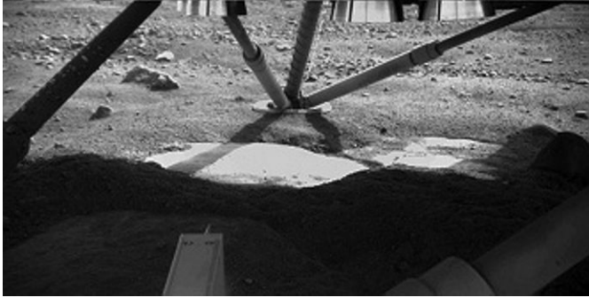
Fig. 7.7. The Robotic Arm Camera captured this image underneath the lander on the fifth Martian day of the Phoenix mission. Descent thrusters on the bottom of the lander are visible at the top of the image. This view from the north side of the lander toward the southern leg shows smooth surfaces cleared of overlying soil by the rocket exhaust during landing. The abundance of excavated smooth and level surfaces adds evidence to a hypothesis that the underlying material is an ice table covered by a thin blanket of soil. The bright-looking surface material in the center, where the image is partly overexposed, may not be inherently brighter than the foreground material in shadow. The Phoenix Mission is led by the University of Arizona, Tucson, on behalf of NASA. Project management of the mission is by NASA's Jet Propulsion Laboratory, Pasadena, California. Spacecraft development is by Lockheed Martin Space Systems, Denver. Image ID 20080531.html, courtesy NASA/JPL-Caltech/University of Arizona/Max Planck Institute.
