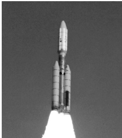
Fig. 4.1. Voyager 1 rides a Titan III-E launch vehicle with Centaur upper stage, leaving Earth half a month after its twin, Voyager 2 . Image courtesy NASA-KSC.
