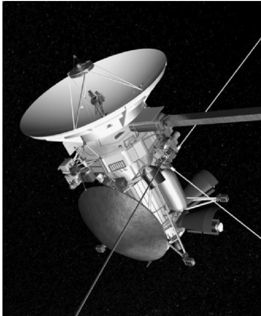
Fig. A.12. Artist's rendering of Cassini spacecraft in flight configuration, shown without blanketing. Three Radio and Plasma Wave (RPWS) antennas extend 10 meters, magnetometer (MAG) boom extends 11 meters. Note the complex of feed horns in the middle of the 4-meter diameter High-Gain Antenna (HGA), which permits the synthetic aperture radar to acquire five parallel image swaths. RTGs are equipped with shades to avoid IR glare in the optical instruments. The Huygens Probe is attached at left, and the optical instrument apertures point toward the upper right. Cosmic Dust Analyzer instrument is the drum near the image's center, and a helium tank for bipropellant pressurization is visible to its lower right. See also: www.jpl.nasa.gov/basics/cassini . Image © Gordon Morrison, reproduced by permission.
