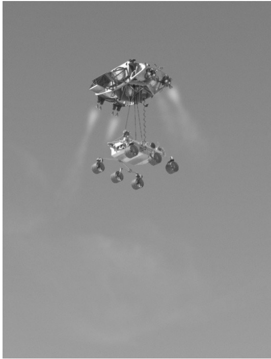
Fig. A.20. Artist's conception showing the Mars Science Laboratory spacecraft being let down to a soft landing by its sky-crane after aerodynamic entry with S-turns, parachute descent, and retro-stage activation. Image courtesy NASA/JPL-Caltech.
