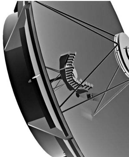
Fig. B.3. Close-up of Cassini Radar multiple feeds near center of HGA used to acquire synthetic-aperture imaging data in five distinct beams. Radar electronics box is mounted atop the bus beneath HGA. Image courtesy NASA/JPL-Caltech.
