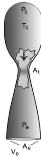
Fig. 4.2. de Laval nozzle. Gas goes supersonic at throat then expands. Notations discussed later in the text.
