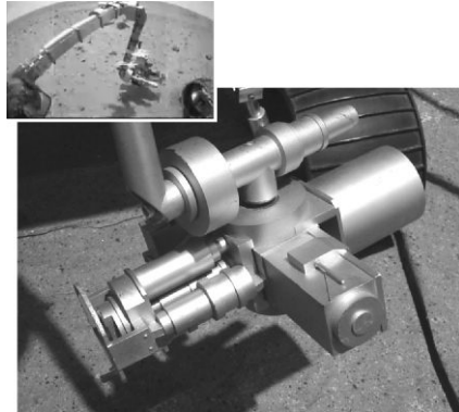
Fig. B.10. Mössbauer spectrometer sensor head is one of four units at the end of robotic arm. Inset: view from mast-mounted NavCam as arm extends toward target on Mars. MIMOS-II is at center in close-up, its aperture represented by concentric discs (APXS is on right, micro-imager behind MIMOS-II, RAT on left). NavCam image and instrument mockup on full-scale model courtesy NASA JPL-Caltech.
