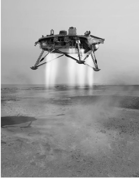
Fig. A.18. Artist's conception of the Phoenix lander spacecraft. Having completed a ten-month journey, the spacecraft's cruise stage was jettisoned five minutes prior to atmospheric entry, then the aerobraking heat shield was released after parachute deployment. When on-board radar sensed it was down to 570 meters above the surface, the parachute was released and hydrazine thrusters carried it to a soft landing as seen here. Loss of sunlight in the winter, extreme cold, and carbon dioxide frost will prevent further operations by January 2009, and there is little chance Phoenix will survive the winter. See also page 269. Image courtesy NASA/JSC.
