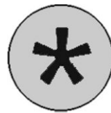
Fig. 4.3. Solid rocket motor cross section. Grey represents the solid propellant molded within the motor casing. The black star represents the cavity in the propellant that serves as combustion chamber.
