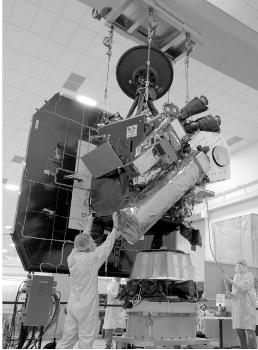
Fig. A.22. Deep Impact flyby spacecraft (above) being mated with the impactor spacecraft (shoulder-level). The impactor operated on battery power after separation, obtaining images and navigating autonomously via built-in hydrazine thrusters, to an impact with the comet at 10.2 kilometers/second. The impact released about 19 gigajoules (equivalent to 4.8 tons of TNT). It returned images on approach via its S-band radio link with the flyby spacecraft. Image courtesy NASA/JSC.
