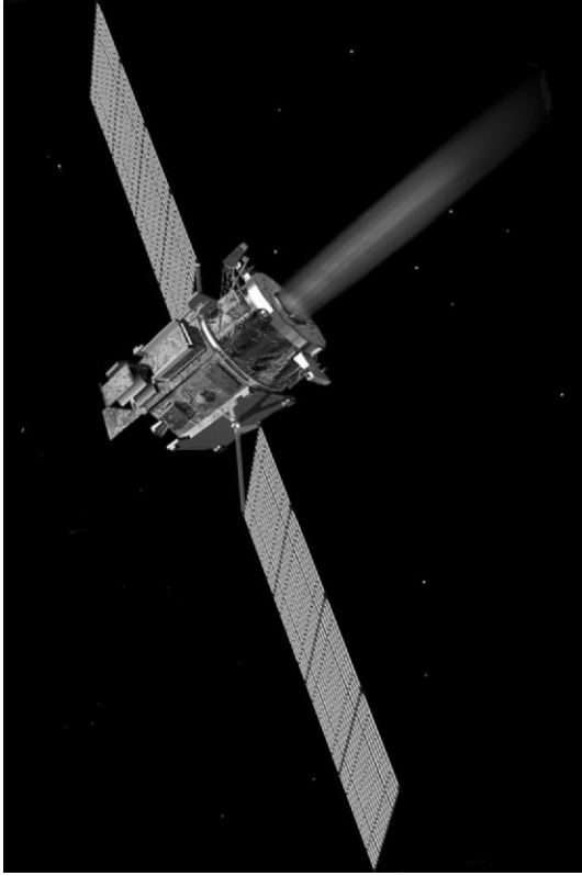
Fig. A.24. Artist's conception of the Deep Space 1 spacecraft in flight configuration operating its solar-electric-powered ion engine. The solar arrays measure about 12 meters end-to-end across the spacecraft. Image courtesy NASA/JPL.
