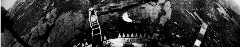
Fig. 6.16. The Soviet Venera 13 spacecraft returned this image of the Venusian surface east of Phoebe Regio in the planet’s equatorial region. Image calibration target is visible on the right. A drilling arm gathered samples for the onboard X-ray fluorescence spectrometer to analyze. Image courtesy NSSDC/GSFC.
