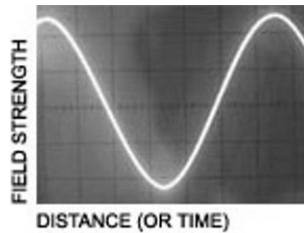
Fig. 1.4. Radio frequency describes how often the cycles of an electromagnetic wave repeat, as the strength of its magnetic or its orthogonal electrical field component increases, decreases, then increases back again. Wavelength is the distance between crests of the wave as it propagates through space.
