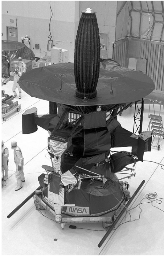
Fig. A.10. Galileo spacecraft. Science boom, folded downward, is left of center with end of stowed MAG boom just left of the NASA emblem. Low-gain antenna No. 1 is atop the stowed central mesh high-gain antenna. Large black circular component is bus sunshade. The heavy ion counter with its two circular apertures, obscured in the drawing on the previous page, is visible atop the bus to the right of center. Three of four hoist attachments, removed before flight, are visible protruding through sunshade. Image courtesy NASA/JSC.
