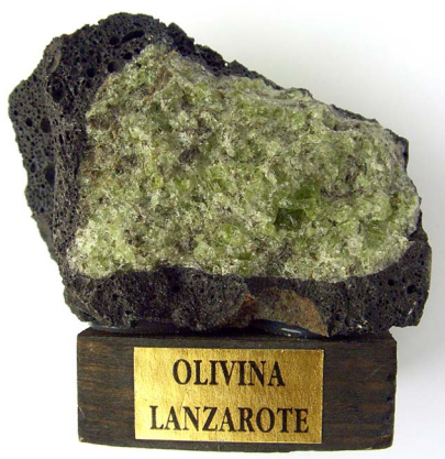
Picture 4.1: The green nodule is enclosed in solidified basaltic lava. The nodule, that comes from the mantle, consists of the ultramafic rock type called peridotite. The dominant minerals in this peridotite are pale green magnesium-rich olivine and lesser amounts of darker green chromium-rich clinopyroxene. The sample comes from Lanzarote, one of the Canary Islands.
