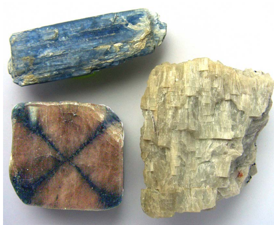
Picture 4.4: Top left: blue kyanite; right: white sillimanite; bottom left: andalusite with a cross-structure (chiasolite).
