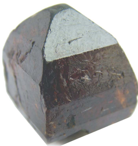
Picture 4.3: Zircon crystal illustrating its tetragonal crystal structure with prism and two types of pyramid faces developed (see also Fig. 3.21).
