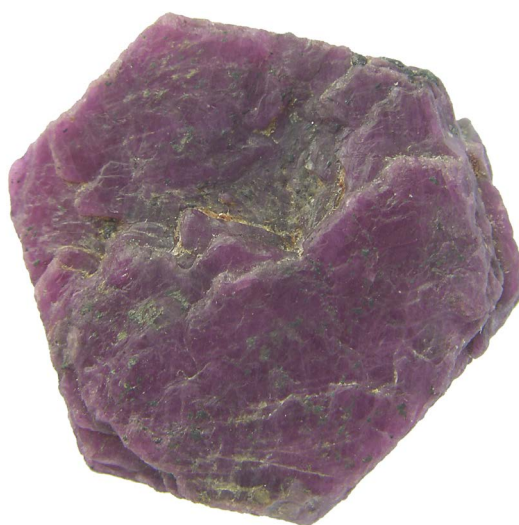
Picture 4.11. Corundum forms 6-sided (hexagonal) crystals. The reddish variety illustrated here is used commercially as ruby.
