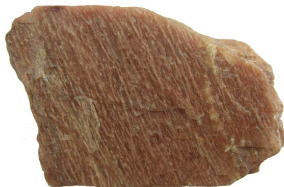
Picture 4.9: Alkali feldspar with well-developed perthite structure. The pinkish host phase is rich in orthoclase (C in Figs. 4.12 & 4.13) whereas the whitish veins are rich in albite (B in Figs. 4.12. & 4.13).
