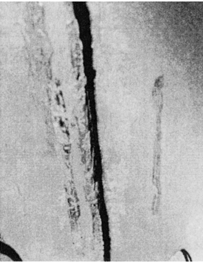
Figure 3-47. Damage to Valve Body Guide Ribs Resulting from Attempted Closure of Wedge Gate Valve with Rotated Wedge Jammed in Valve Body, Size DN 300 (NPS 12) Class 150. (Courtesy of David Mair.)
