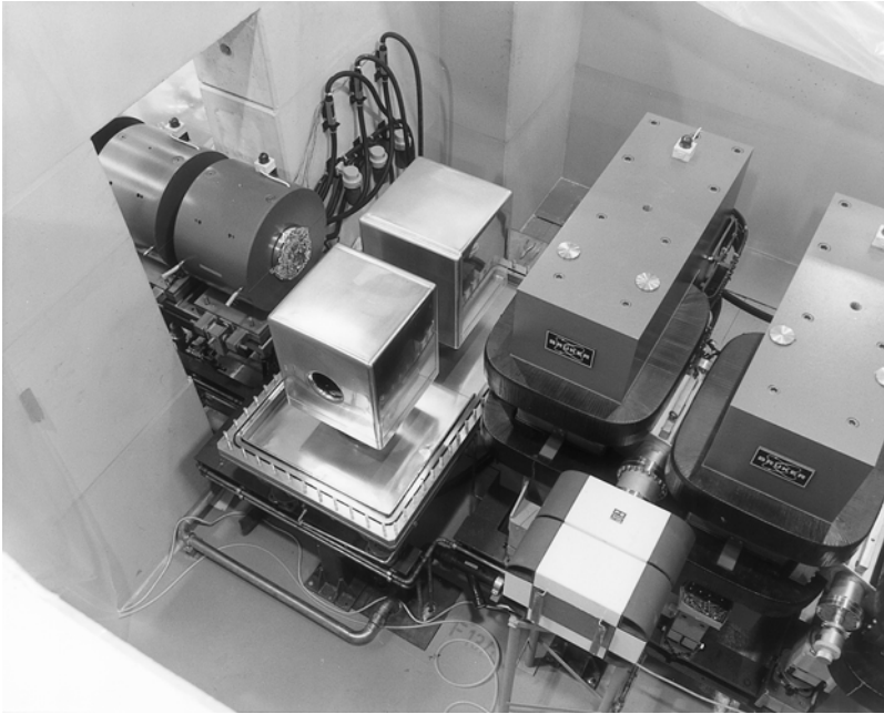
Figure 9.4 Photograph showing the main parts of the velocity filter SHIP. From the left: 1, two quadrupoles of the first quadrupole triplet; 2, two cubes for the creation of an electric dipole field. The cubes are charged up to voltages of about +100,000 Volts and -100,000 Volts, thus creating a strong electric field between the plates which are 15 cm apart. The vacuum vessel above the two cubes was removed; 3, two of the four dipole magnets. These are electric magnets and we can see the isolation of the copper coils surrounding the iron. A current of about 100 Amperes creates the necessary magnetic field strength.
