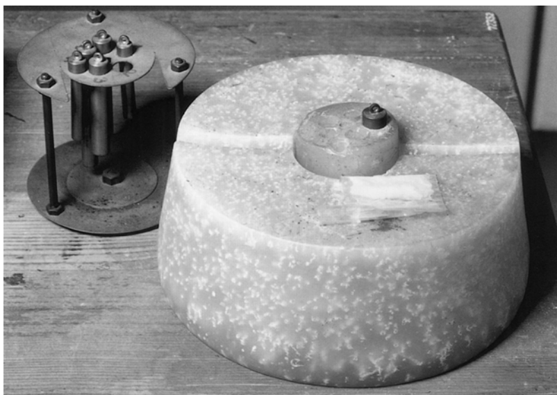
Figure 3.1 Neutron sources (left) and paraffin moderator used by Otto Hahn in experiments for the synthesis of transuranium elements which resulted in the discovery of fission. The figure was taken from History of the discovery of nuclear fission , Technical University Berlin, 1989.
