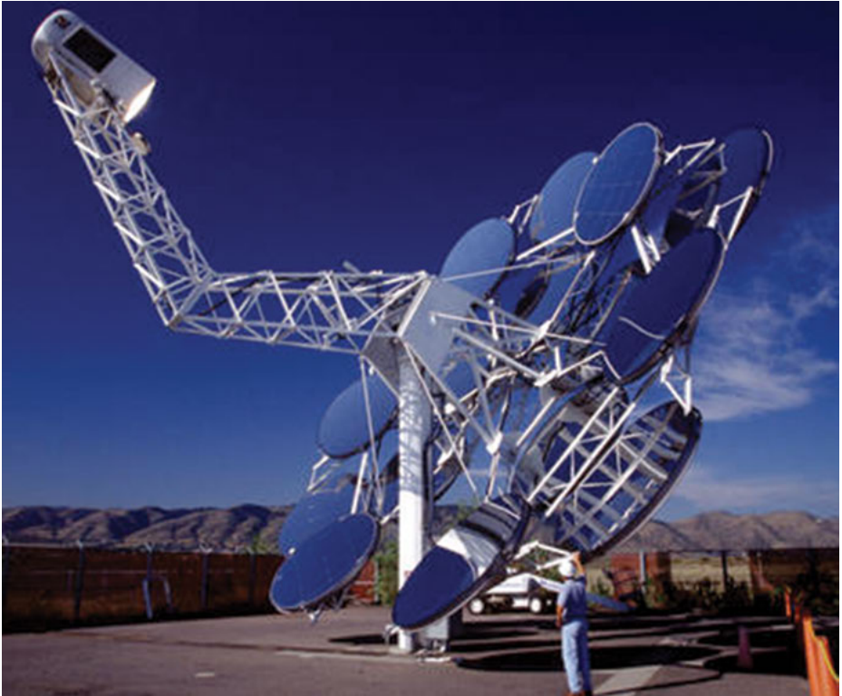
Figure 8.6: Stirling engine CSP. (Photo, public domain, courtesy of the National Renewable Energy Laboratory)
