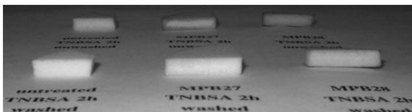
Figure 12.8 Left to right: untreated, \text{NH}_3 plasma-treated (continuous-wave), and pressure pulsed \text{NH}_3 plasma-modified porous polypropylene membrane material. The \text{NH}_2 groups formed were colorized by reaction with 2,4,6-trinitrobenzenesulfonic acid.
