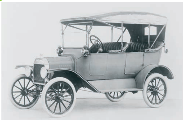
Figure 4.19 Henry Ford came across a vanadium alloy in 1905 in a crash at a racing event. When Ford picked up a fragment, which was part of a valve spindle, he was surprised how strong it was. He decided his new Model-T car would be made from vanadium steel. Mass production began in 1913 and 15 million cars were made, all with vanadium steel components.
