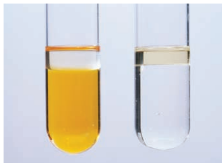
Figure 14.42 Orange bromine water is decolourised by an alkene but remains unchanged in the presence of an alkane.
