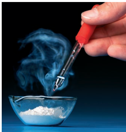
Figure 4.6 The reaction between calcium oxide and water is the reaction used in self-heating coffee cans (Figure 4.3). It is a vigorous reaction and here, steam is seen rising from the hot reaction mixture. The standard enthalpy of reaction for the calcium oxide and water is \Delta_r H^\circ = -63.7 \text{ kJ mol}^{-1} .
