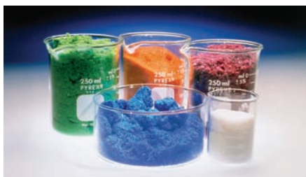
Figure 2.9 Each beaker contains 1 mole of a different coloured compound and hence each contains the Avogadro constant number of particles. The compounds shown are copper carbonate, hydrated copper sulfate, sodium chloride, potassium manganate(VII) and potassium dichromate(VI).
