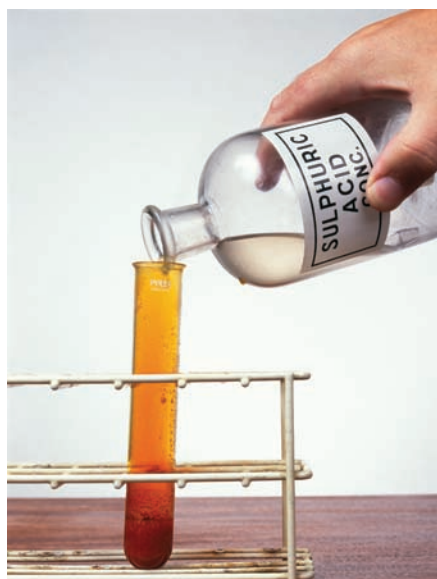
Figure 10.10 Bromine gas forming as the product of a reaction between concentrated sulfuric acid (in bottle) and sodium bromide (in test tube).
