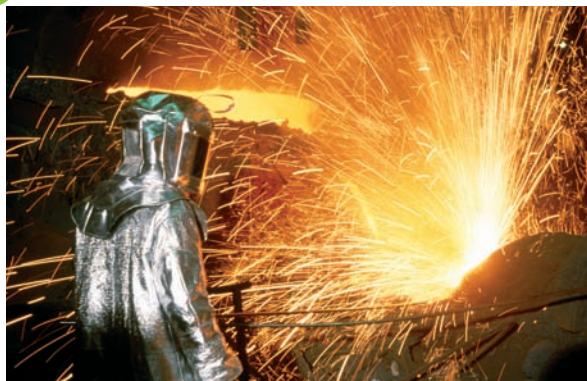
Figure 4.17 Iron is extracted from its ore in a blast furnace. Heat radiated from the metal is reflected away by the shiny surface of the protective suit, which covers all of the body.
