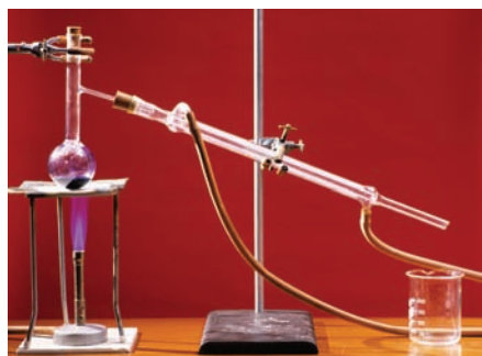
Figure 15.9 Apparatus for oxidation of a primary alcohol to produce an aldehyde.
