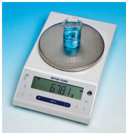
Figure 17.9 A top pan balance is used in the laboratory to measure mass.
