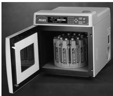
FIGURE 7.4 MARS 5 MAE instrument with open door allowing view of vessels inside. (Courtesy of Elaine Hasty, CEM Corporation, Matthews, NC.)
