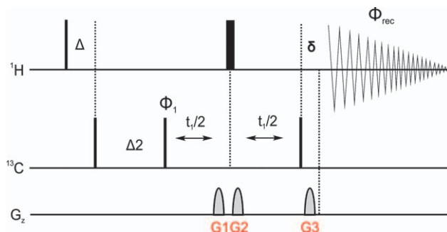
Figure 9.17 The HMBC pulse sequence first described in 1986 by Bax and Summers. 49 The initial 90^\circ ^1\text{H} pulse is followed by a delay, \Delta , and then a 90^\circ ^{13}\text{C} pulse, which serves as the low-pass J -filter to suppress unwanted ^1J_{\text{CH}} doublets flanking the proton chemical shift. The delay should be set to \Delta = 1/2(^1J_{\text{CH}}) ; 145 Hz is generally a good compromise value. The delay \Delta 2 following the first ^{13}\text{C} pulse is the long-range delay, \Delta 2 = 1/2(^nJ_{\text{CH}}) , and should generally be set in the range of \sim 3 –10 Hz. Phase cycling is simple: \Phi_1 = 0, 2 ; \Phi_{\text{rec}} = 0, 2 , and as would be expected, the gradient ratio must be adjusted as a function of the heteronuclei, hence G1 : G2 : G3 = 50 : 30 : 40.1 for ^1\text{H} – ^{13}\text{C} and 70 : 30 : 50.1 for ^1\text{H} – ^{15}\text{N} . No decoupling is applied during acquisition and it is advisable to acquire the data using at least 4K points.
