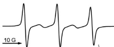
Fig. 16 EPR signal of 7 (0.05 mM) recorded in water at 328 K. Reprinted with permission from C. Casati, P. Franchi, R. Pievo, E. Mezzina and M. Lucarini, Unraveling Unidirectional Threading of A-Cyclodextrin in a [2]Rotaxane Through Spin Labeling Approach, J. Am. Chem. Soc. , 2012, 134 , 19108. Copyright 2012 American Chemical Society.
