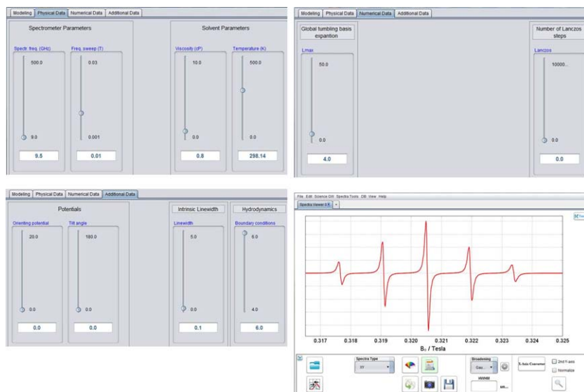
Fig. 8 VMS panels showing the various input data to be set. The calculated spectrum is shown in the lower right panel.
