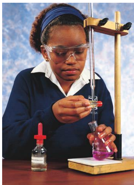
Figure 8.13 The acid is added to the alkali until the indicator just changes colour.
