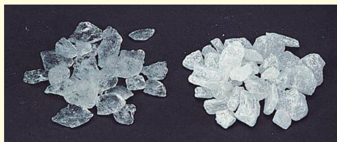
Figure 8.22 A white powder forms on the surface of sodium carbonate decahydrate when it is left in the air.
