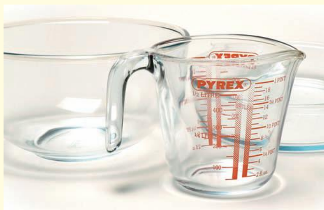
Figure 3.38 This glassware is made from Pyrex, a heat-resistant glass.
