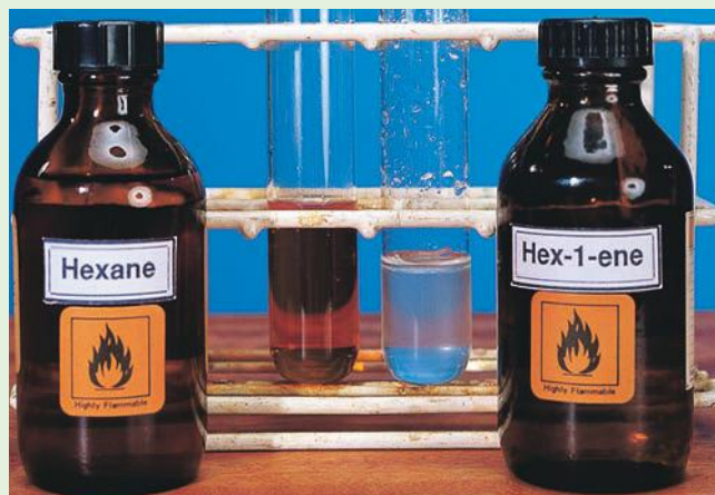
Figure 14.13 The alkene decolourises bromine in 1,1,1-trichloroethane.
