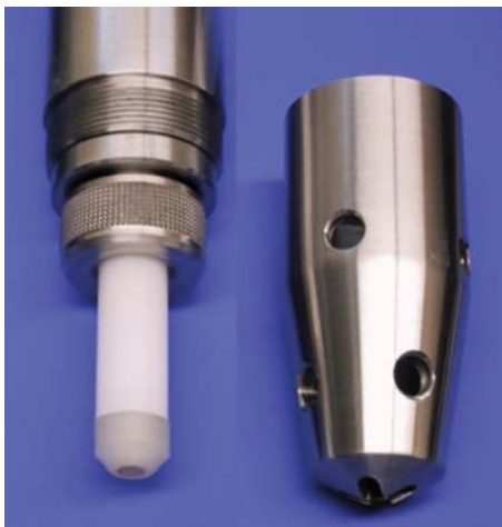
Figure 12.17 CO 2 probe with unscrewed protective cap (KSI Meinsberg) for measuring the CO 2 content of the water at the bottom of a borehole.
