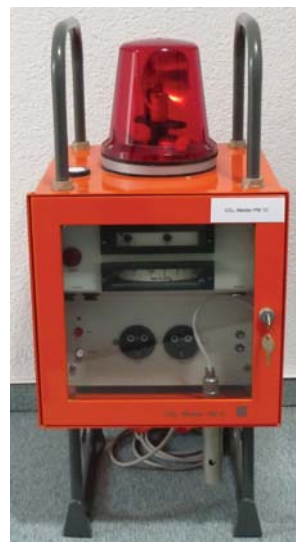
Figure 13.3 Stationary CO 2 warning device with electrochemical CO 2 sensor for application in underground potash salt mining. Source: KSI Meinsberg.
