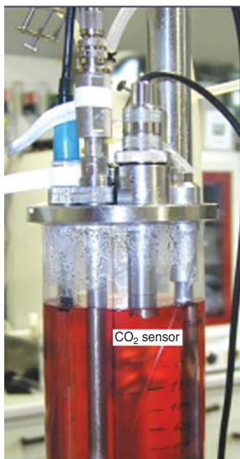
Figure 14.2 Two litres stirred bioreactor (VSF 2000, Bioengineering AG, CH) with electrochemical carbon dioxide sensor (KSI Meinsberg Kurt Schwabe Research Institute, Germany).
