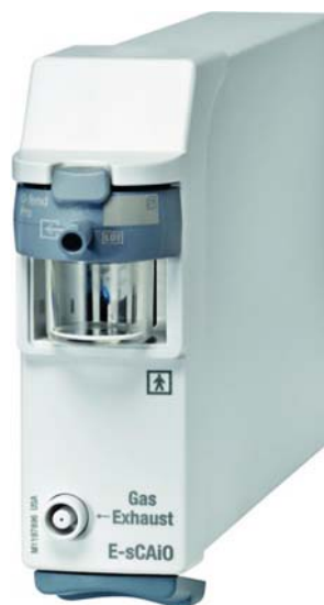
Figure 16.7 Capnograph with one compact module for respiratory monitoring of O 2 , CO 2 , and N 2 O, anaesthetic agents sucking the breathing gas sample with 120 ml min -1 by the side-stream method (GE Healthcare). Courtesy Reference.
