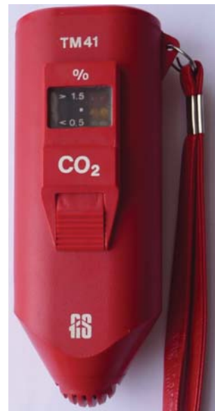
Figure 13.2 Portable CO 2 warning device with electrochemical CO 2 sensor. Source: KSI Kurt-Schwabe Research Institute Meinsberg, Germany.
