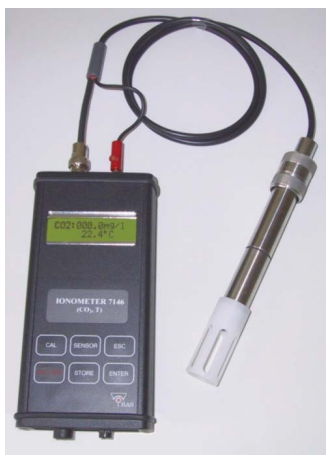
Figure 15.2 Electrochemical carbon dioxide sensor and handheld CO 2 metre [5].
