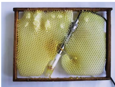
Figure 15.8 Electrochemical carbon dioxide sensor (EMCO2, KSI Meinsberg) in a honeycomb. Source: Zosel et al. 2011 [52]. Reproduced with permission of IOP Publishing.
