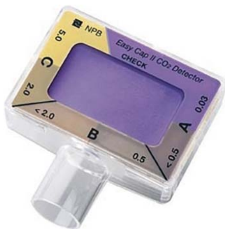
Figure 16.5 Colorimetric sensor for CO 2 analysis in breath (Nellcor™ adult/pediatric colorimetric CO 2 detector). This single-use sensor provides direct visual feedback of the exhaled CO 2 in a semi-quantitative way through a colour change from purple (in the black/white figure dark gray) to yellow (in the black/white figure light gray in the upper left corner).
