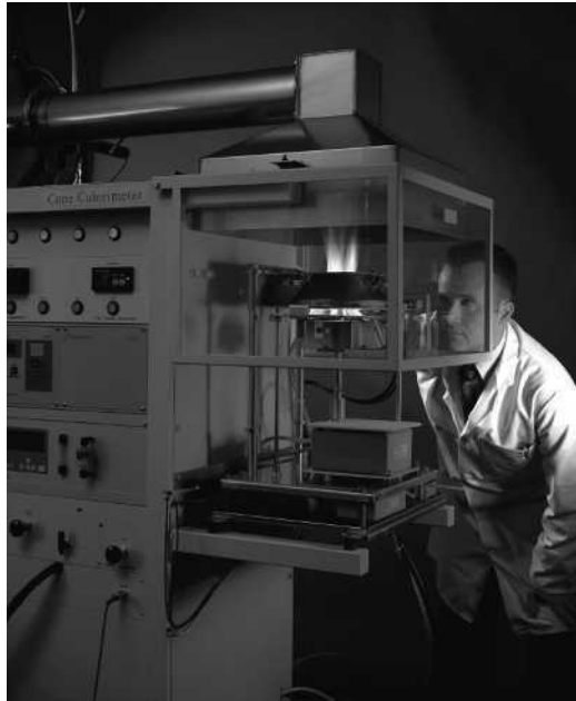
Figure 5.10 Cone calorimeter test. Reproduced with permission from Fire Testing Technology Limited, East Grinstead, West Sussex, UK
