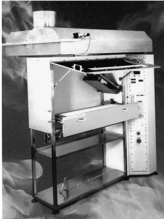
Figure 5.4 Flooring radiant panel test method. Reproduced with permission from Fire Testing Technology Limited, East Grinstead, West Sussex, UK
