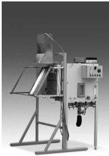
Figure 5.3 ASTM E162 [4] radiant panel test method. Reproduced with permission from Fire Testing Technology Limited, East Grinstead, West Sussex, UK
