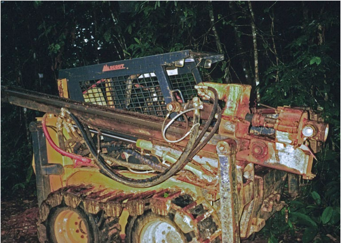
Figure 2 Closeup of rubber-tired, self-propelled combination diamond, reverse circulation and auger drill (Scout). Reproduced with permission from CRC Press / Balkema. (See insert for color representation of the figure.)
