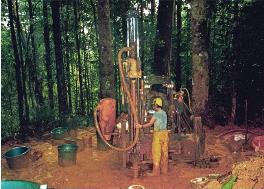
Figure 1 Tracked and tired lightweight drill in operation. Reproduced with permission from CRC Press / Balkema
