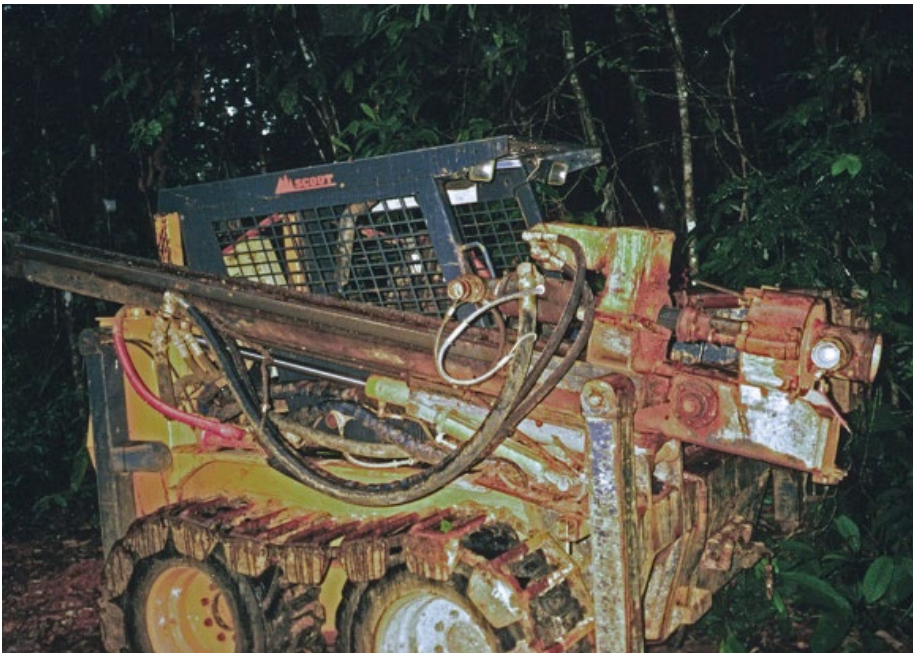
Figure 2 Closeup of rubber-tired, self-propelled combination diamond, reverse circulation and auger drill (Scout). Reproduced with permission from CRC Press / Balkema
