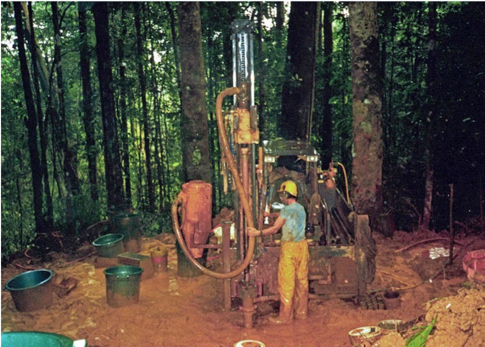
Figure 1 Tracked and tired lightweight drill in operation. Reproduced with permission from CRC Press / Balkema. (See insert for color representation of the figure.)
