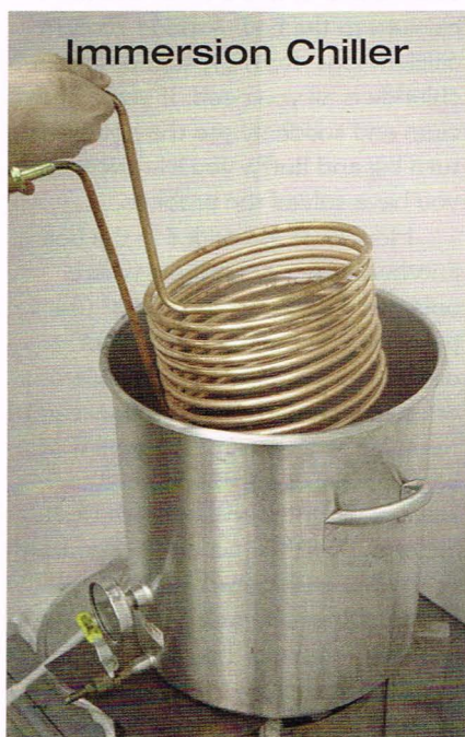
An immersion chiller is a heat exchanger that will rapidly cool the wort.
