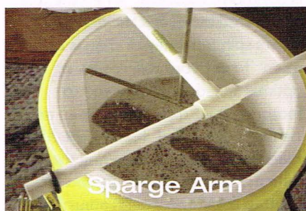
Sparge water is used to rinse the grain bed, to get a better yield from the malts.
