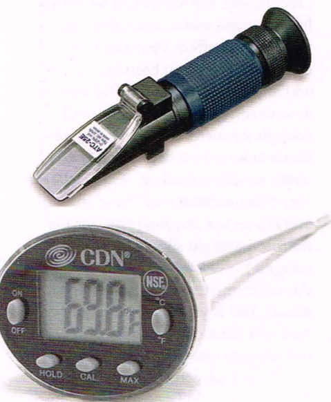
A refractometer (top) and digital thermometer. Both should be calibrated before use.
