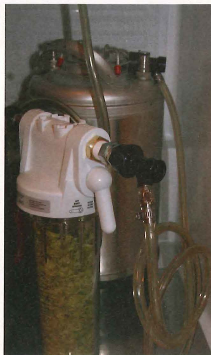
This hop filter project is an easy way to make your kegged homebrew much hoppier.
