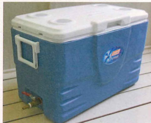
A Coleman Xtreme cooler makes an excellent mash tun with a few copper pipe and fittings modifications.
