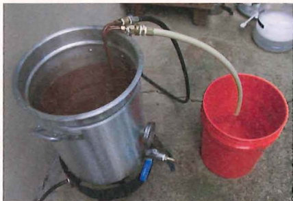
A copper immersion chiller will quickly cool the wort after the boil.
