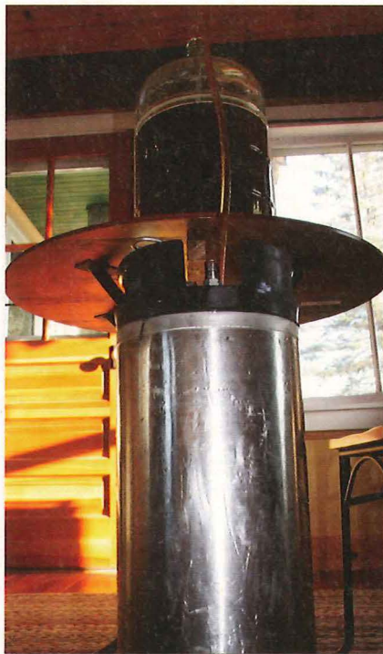
To siphon, the container filled with beer needs to be higher than the empty vessel.
