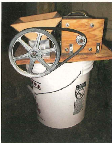
Steve made this motorized mill with a washing machine motor for less than $30.
