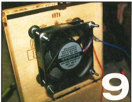
A hole drilled in the back of the box accepts the power cord (Figure 8). Washers provide space between the fan and the box (Figure 9).
