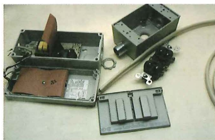
With the duplex box disassembled, screw in the close nipple and open the controller.
