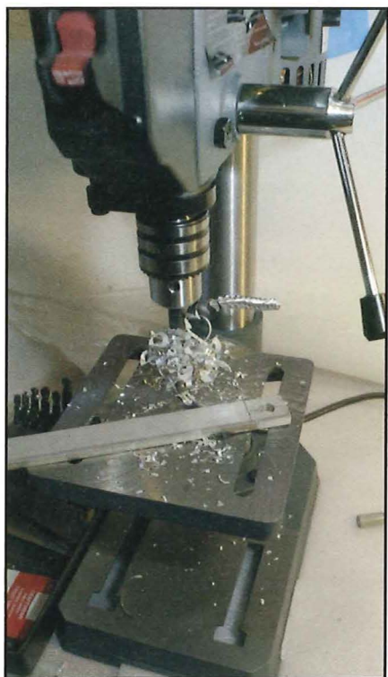
You will need to drill a 1/2-inch opening for the male adapter. (Hint: medium pressure, low speed and titanium drill bits work best for stainless steel.
