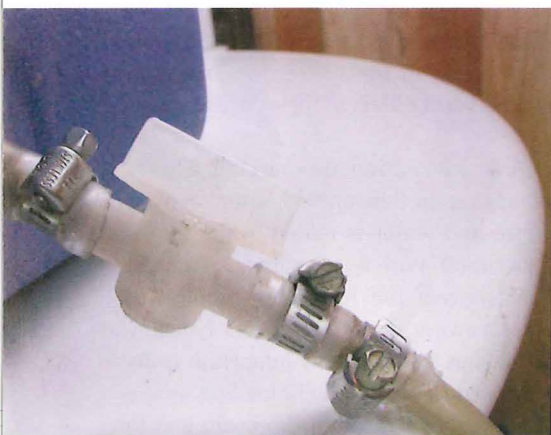
A stainless steel braid (picture at right) separates the wort from the grains. It is made from a water supply line. A valve on the outside of the cooler (above) regulates the outflow of wort.
