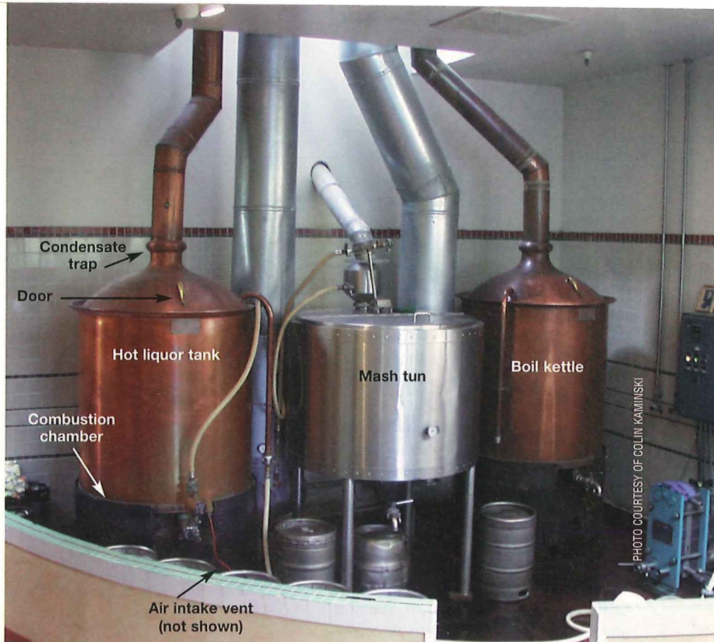
Above: The brewing system at Downtown Joe's in Napa, California, where author Colin Kaminski works. It's an enclosed system with a combustion chamber. Left: A homebrew system that'll be fired by propane piped in from outside, with an exhaust hood and fan.
