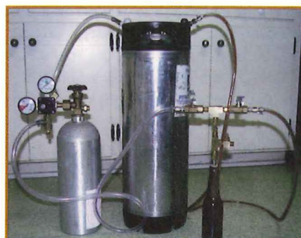
You'll need a keg and a carbon-dioxide cylinder to connect to your counter-pressure bottler.
