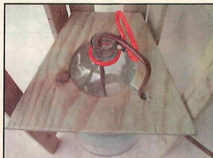
Looking at the underside shows how the carboy's neck fits in the collar and the spray wand extends into the carboy.
