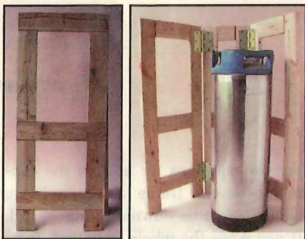
The sides are hinged, making this CIP device adjustable and easy to store.
