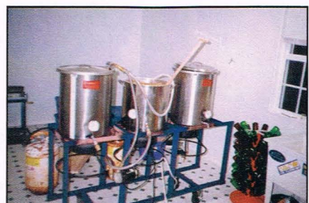
Three gas burners, stainless-steel pots, a stand and a bottle drying rack.
