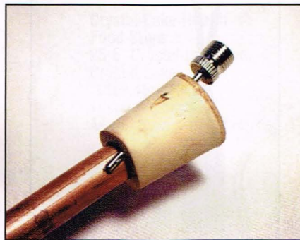
You also push the needle through the hole you drilled in the stopper.
