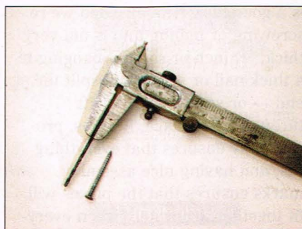
The plywood is not very thick, so make sure your screw or nail isn't too big.
