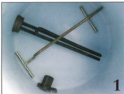
The Chromalox heating element is protected by a vertical standoff made from a bent 1/4-inch brass welding rod.
