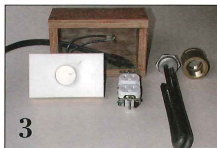
The Chromalox heating element and controller parts: light dimmer, electrical outlet and a two-wire power cord.
