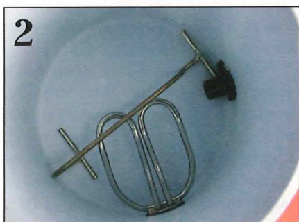
The Cordon Brew heating element under the standoff, which protects the element and supports the mash screen.
