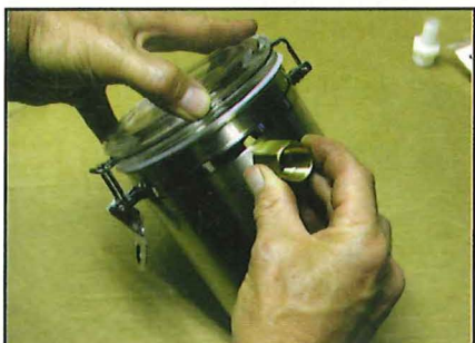
Measure the hole locations, leaving enough room at the top and bottom.
