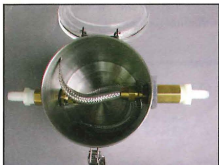
The final product: Note the bulkhead fittings for both the inlet and outlet.
