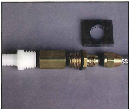
The input fitting: All the parts you need to assemble the top bulkhead.
