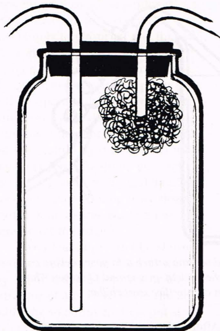
Mason Jar: The "wort-in" nipple has copper tubing that extends to the bottom of the jar. The "wort-out" nipple has a short tube protected by a Choreboy.
