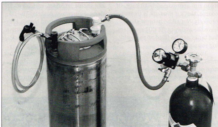
First draft: This is a standard set-up. It has a Cornelius keg to hold the beer, a carbon-dioxide tank, a two-gauge regulator and a "cobra head" tap.
