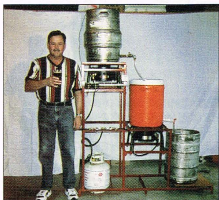
I built a three-tier all-grain system and added two handy temperature gauges.
