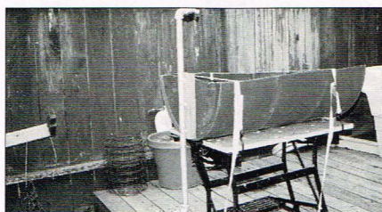
Dianda cut a 55-gallon malt drum in half to make this portable brewing sink. He soaks bottles in the other side.
