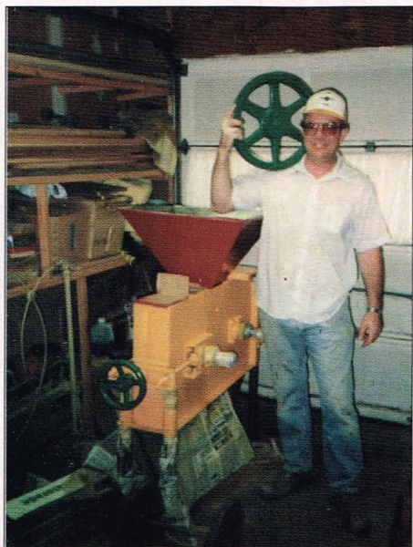
The "Missing Link" grain mill came from a Nebraska hog farm. Ken Piels refurbished it for use in the brewery.
