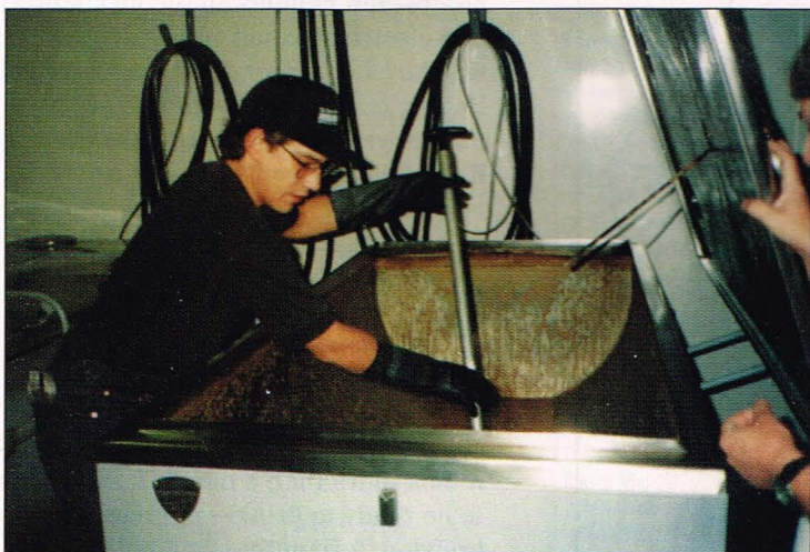
Jim Dallarosa cleans one of the original fermentation tanks, which were converted from dairy equipment.
