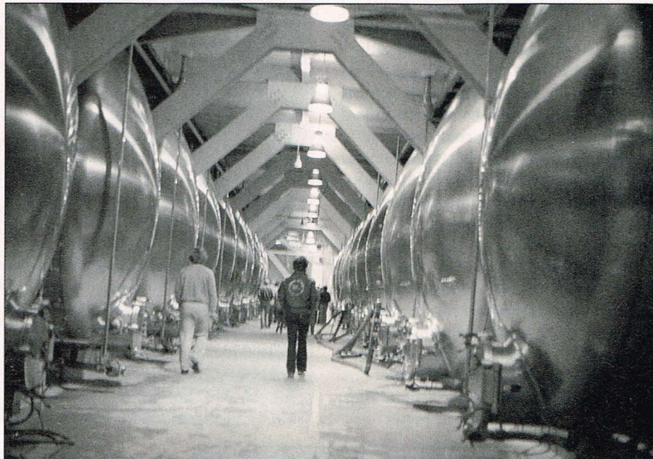
Giant lagering tanks at Anheuser-Busch keep beer near freezing during lagering.
