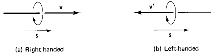
Figure 4.9 Helicity. In (a) the spin and velocity are parallel (helicity +1 ); in (b) they are antiparallel (helicity -1 ).
