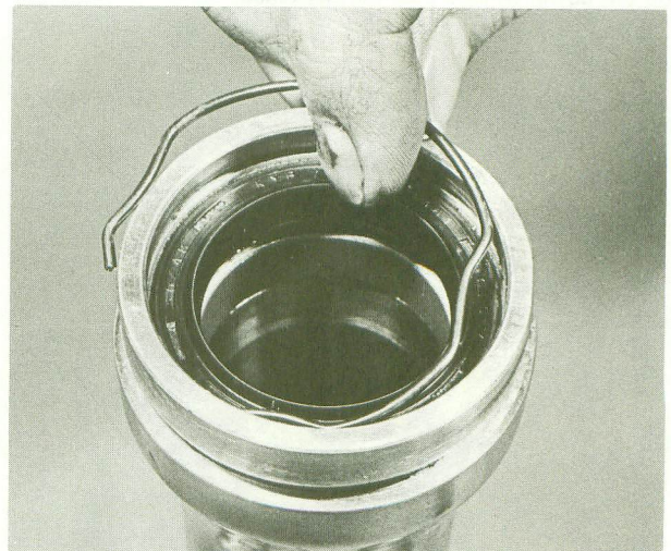
12.7d Fork oil seal is located by a wire retaining clip
