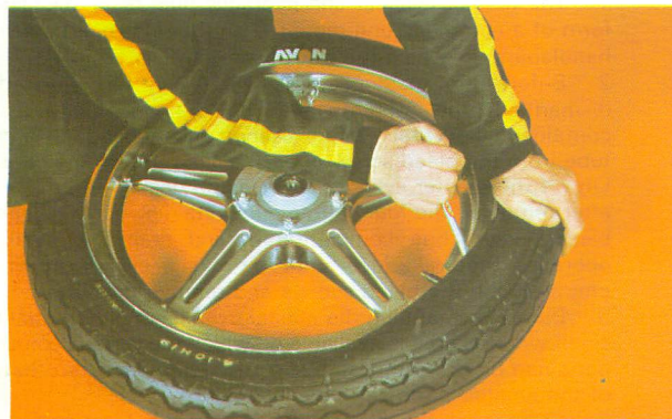
Use lever in final section
