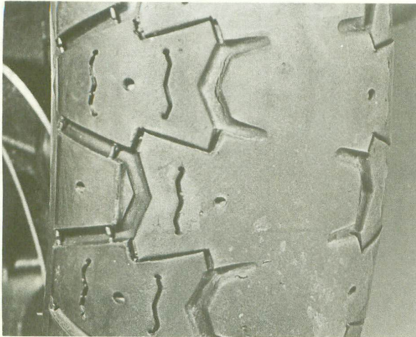
In the case of this tyre, a tread depth gauge was unnecessary. This tyre is dangerous, and in many areas, illegal
