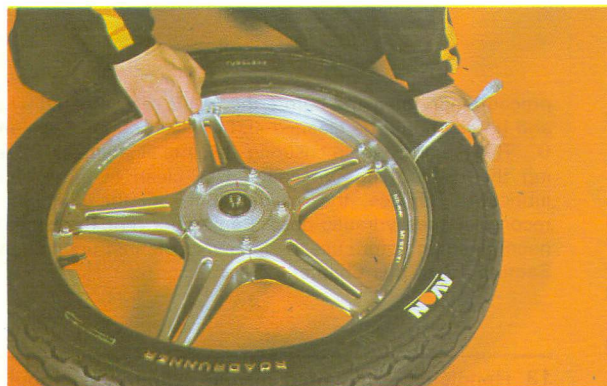
Start second bead under the rim opposite the valve
