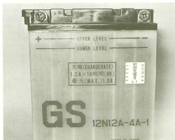
6.2 Battery electrolyte level is visible through translucent case
