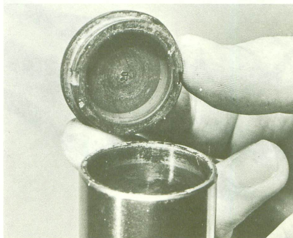
12.1 Remove plastic cap from top of stanchion
