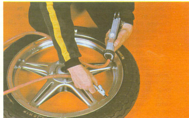
Air hose may be required for initial tyre inflation
