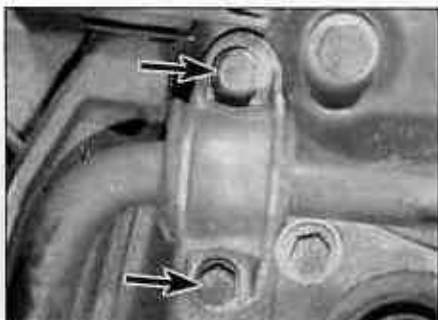
4.2b ... and the suspension sub-frame (arrowed)
