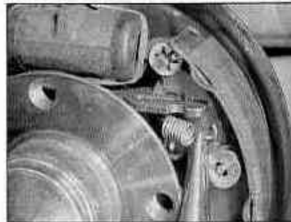
5.7a Unhook the self-adjuster mechanism from the trailing shoe ...
