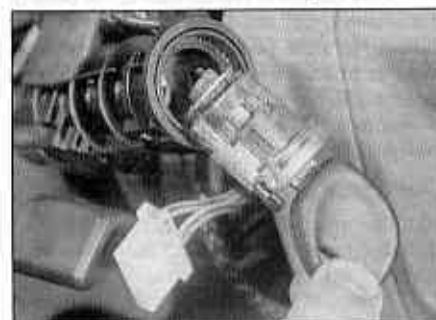
10.5b Depress the release button and withdraw the lock cylinder
