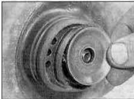
3.8a Withdraw the washer . . .
