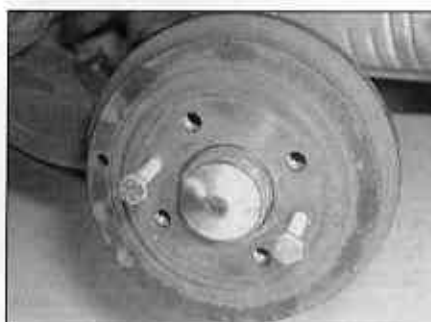
6.3 Using two bolts to draw the drum off the brake shoes
