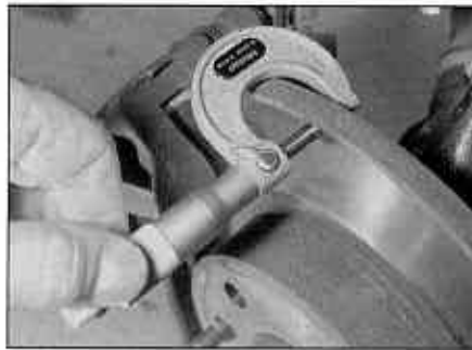
4.8 Measuring brake disc thickness with a micrometer
