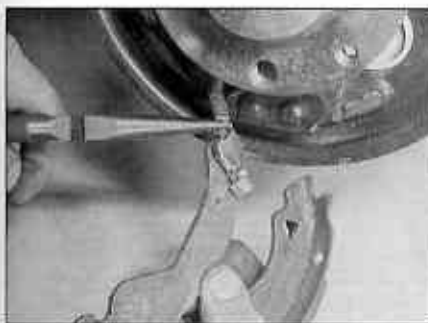
5.8c ... and disconnect the handbrake cable from the brake shoe lever
