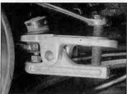
17.2a Balljoint separator tool in use on the track-rod end
