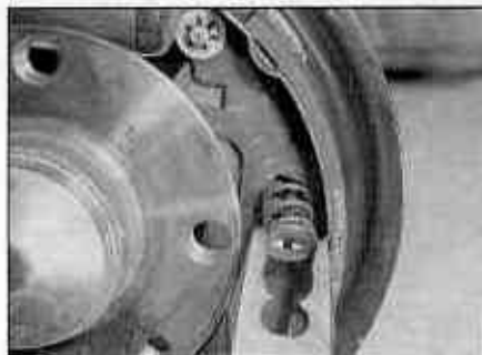
5.8a Remove the hold-down cup and spring from the trailing shoe
