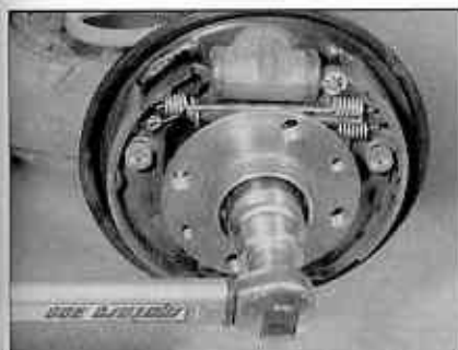
7.5 Slacken and remove the rear hub nut
