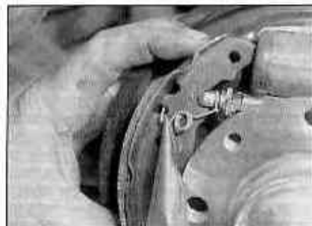
5.5 Unhook the self-adjuster mechanism return spring from the leading brake shoe
