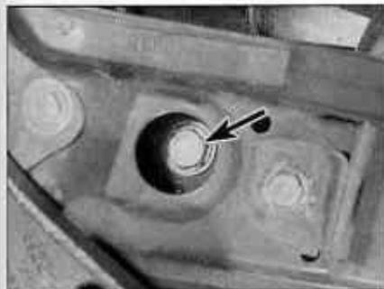
13.11b ... and left-hand steering gear-to-subframe bolts
