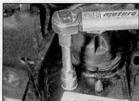
3.18 Fit the strut upper mounting bolts, and tighten them to the specified torque
