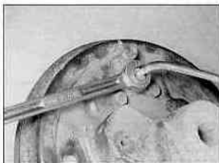
7.4 Unscrew the union nut and disconnect the hydraulic pipe from the rear of the wheel cylinder
