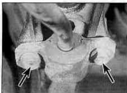
4.2a Unscrew the bolts (arrowed) securing the anti-roll bar mountings to the suspension lower arms ...
