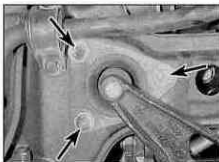
12.9 Unbolt the rear engine mounting-to-subframe bolts (arrowed)
