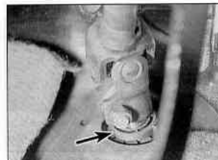
11.6 Slacken the nut (arrowed) and clamp bolt on the lower half of the universal joint
