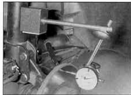
4.11 Brake disc runout measurement - DTI gauge method
