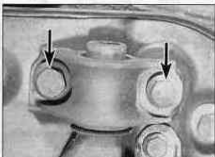
4.4 Unscrew the two bolts (arrowed) and detach the suspension arm rear mounting bracket from the subframe
