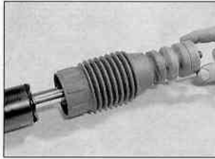
3.9b . . . then withdraw the dust cover and bump rubber
