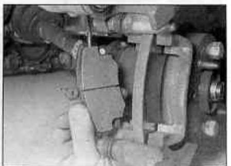
2.8b ... and inboard brake pads from the caliper bracket
