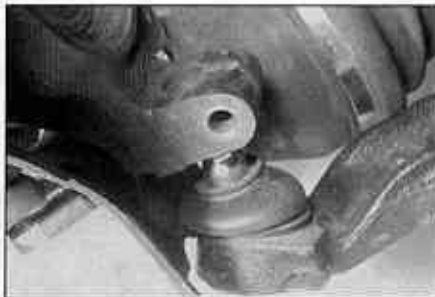
2.8c ... then push the lower arm down and separate the balljoint from the base of the hub carrier
