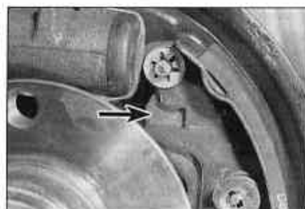
5.12 Fit the self-adjuster mechanism into the recess (arrowed) in the trailing brake shoe
