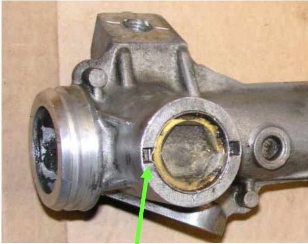
RACK PRELOAD IS STAKED IN PLACE
