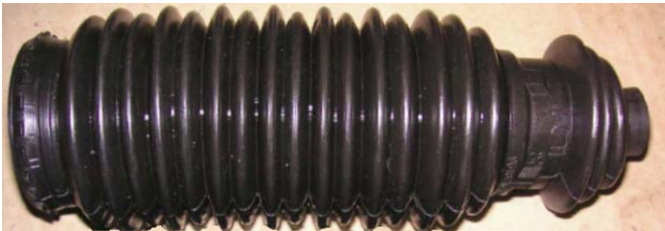
DESPITE APPEARANCES THE RH GAITER IS ONE PIECE.
