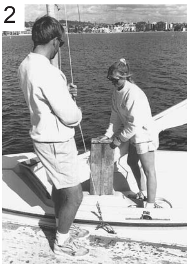
Slide in the daggerboard.
