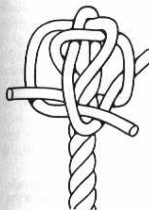
Fig. 118 Smaller rose knot
