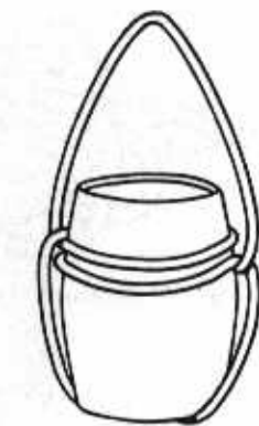
Fig. 151 Sling on a cask
