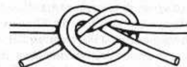
Fig. 95 Ordinary bend or overhand bend
