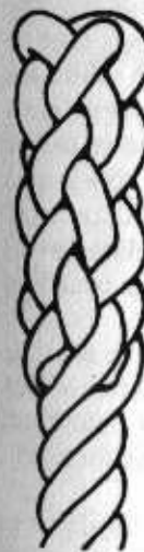
Fig. 33 Back splice or Spanish whipping
