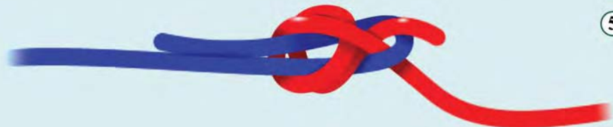
Two lines joined by a double sheet bend.
