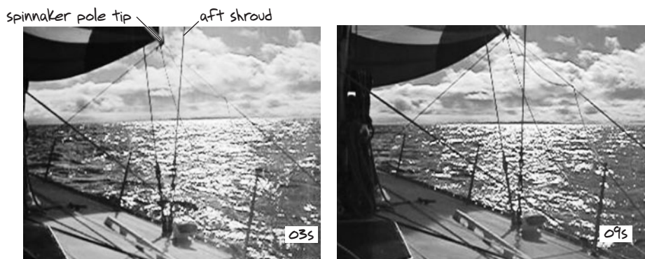
Figure 4-1. Keeping track of a heading relative to clouds. Note the location of the aft shroud relative to the cumulus dome just off the spinnaker pole tip. At 3 seconds, it is just to the left of the dome, and at 9 seconds it is just to the right. Clouds are not permanent references, but this type of alignment is superior to trying to chase a compass card (if you had one) or even a telltale for short-term adjustments.
