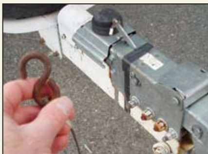
The surge brake breakaway lanyard is designed to be connected from the tow vehicle to the locking actuator lever on the master cylinder.
