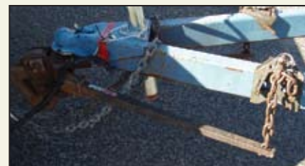
A typical weight-distributing hitch with spring bars. As the bars are tensioned by means of the adjustable chains and lever brackets, the rear of the truck is jacked up. This shifts tongue loads towards the front of the tow vehicle.
