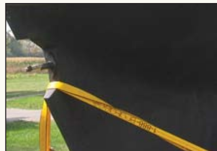
(top) In addition to the fore and aft tie-down straps, a tight ratchet strap to the trailing edge of the keel helps to keep the boat from creeping aft on the trailer. (bottom) On a full-keel boat you'll need to engineer the strap to pass through the propeller aperture.
