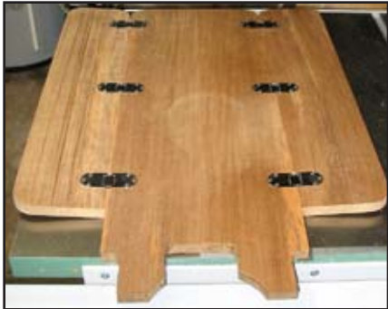
Hinge details: (top) cut the deeper section for the hinge knuckle, then (bottom) check the fit. the wings folded in.
