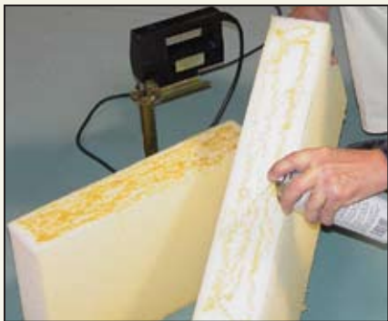
Using 3M Super Trim Adhesive to glue two pieces of foam together.
