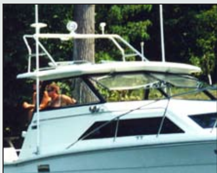
Custom designed and built tube radar arch.
