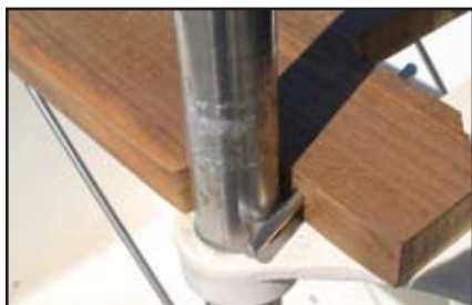
(top) Use extra long bit to drill for holding pins. (bottom) Holding pin positioned in table.
