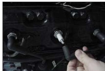
Get a tune-up: routinely inspect spark plugs and wires. Fouled plugs and worn wires burn more fuel.
