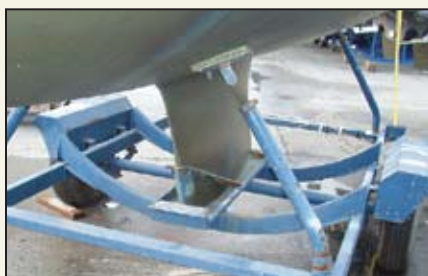
(top) Where is the forward keel brace? (bottom) There it is! This piece can make all the difference as to whether or not the boat remains stationary under emergency braking or in a minor collision.
