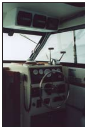
(above) Helm under construction. (across) More functional helm station with vinyl-covered plywood instrument box overhead and a new Formica panel with Faria gauges relocated above the steering wheel.
