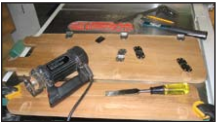
(left) Dry fit the hinges then (right) using a template cut the hinge recesses.
