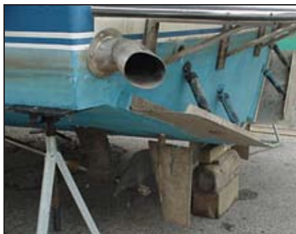
Trim it right. Be sure rudders are aligned and trim tabs are working correctly.
