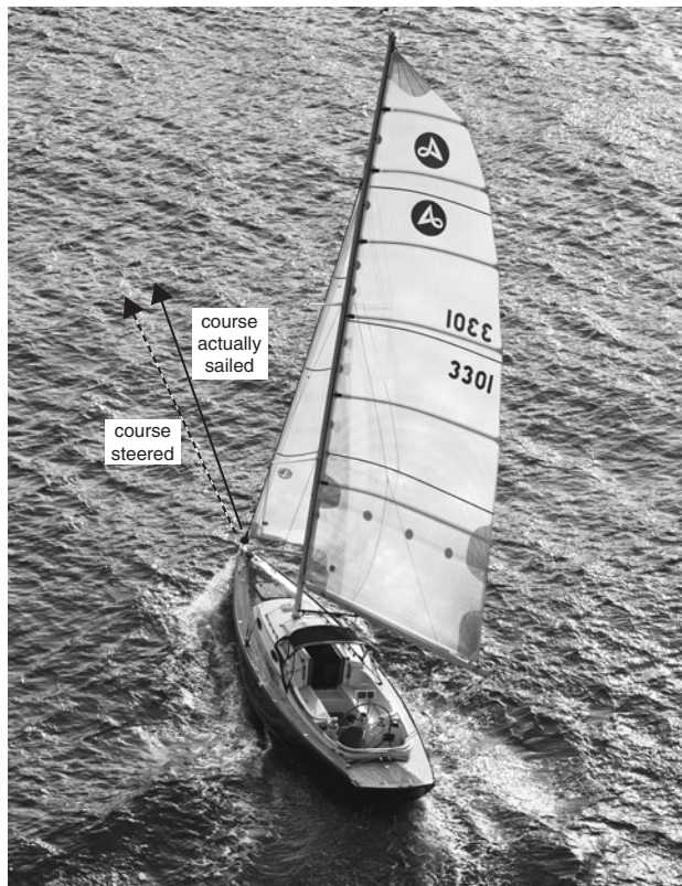
Leeway is the difference between the course steered and the course actually sailed. All boats make leeway, especially when sailing to windward. (Billy Black)
