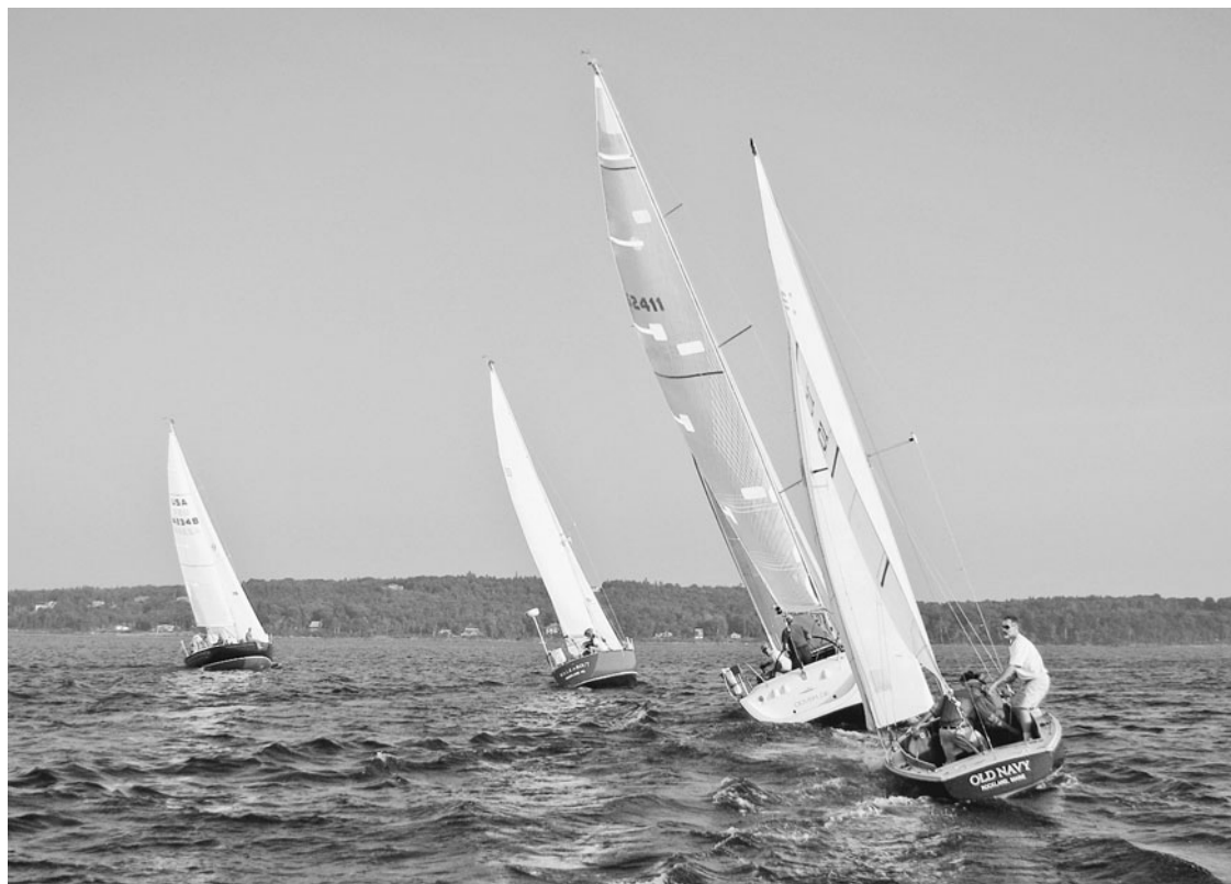
Watching the way another boat has its sails trimmed allows you to infer the wind direction in its area. You can also deduce wind strength by watching the other boat's angle of heel. (Stephen Gross)
