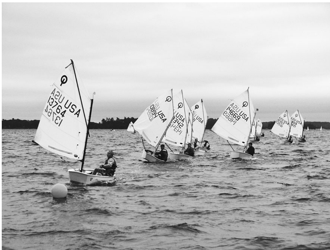
Shifting crew weight to change a boat's angle of heel can have a dramatic effect on boat speed. These Optimist sailors are heeling their boats to windward on the downwind leg of their race course. (Molly Mulhern)
