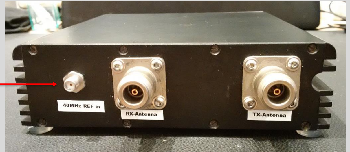
ADALM Pluto in shielded encasing with external 40 MHz reference input
