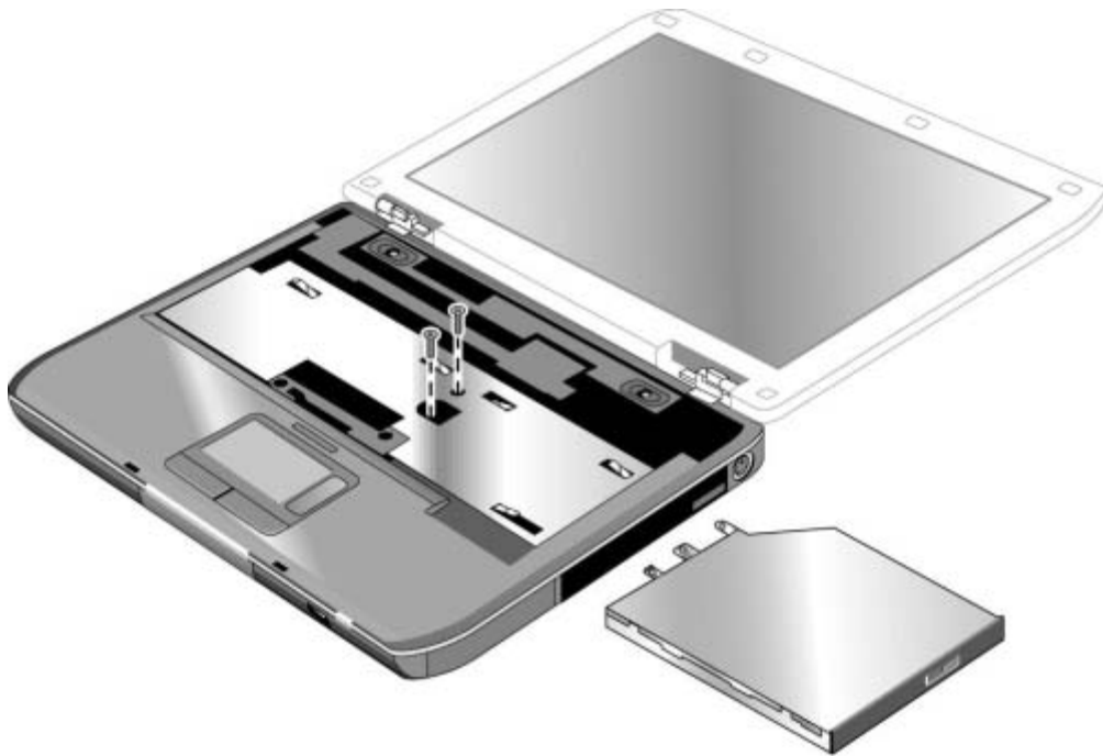
Figure 2-15. Removing the CD/DVD Drive
