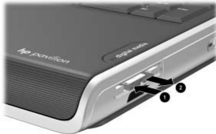
Releasing and removing a digital media card
