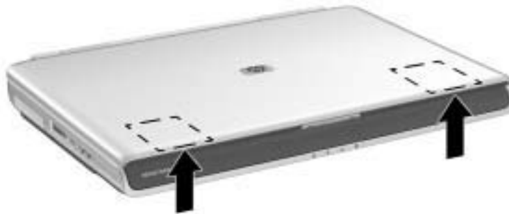
Wireless antennae location
