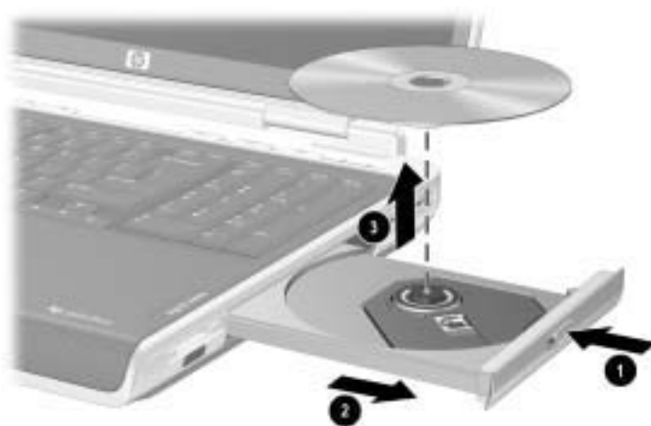
Removing an optical disc from the optical drive when power is available
