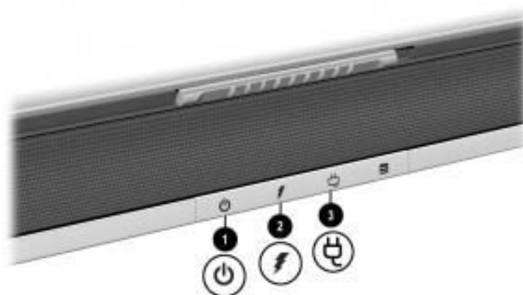
Identifying the battery and power/standby lights
