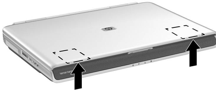
Wireless antennae location
