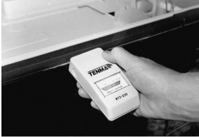
FIGURE 2-22 After repairs, check the oven door for possible radiation leakage.
