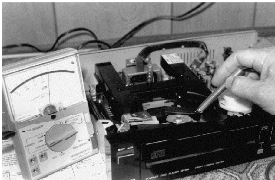
FIGURE 28-2 Check the laser diode with a power meter.
