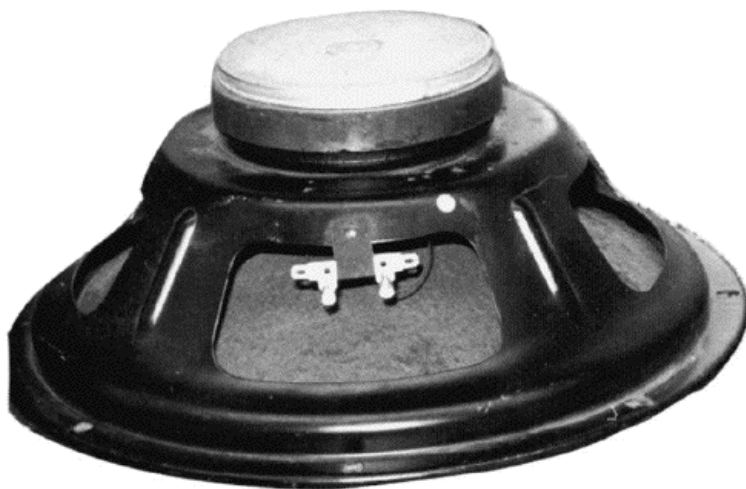
FIGURE 16-30 A dc voltage or excessive volume applied to the voice coil and even damage high-wattage speakers.
