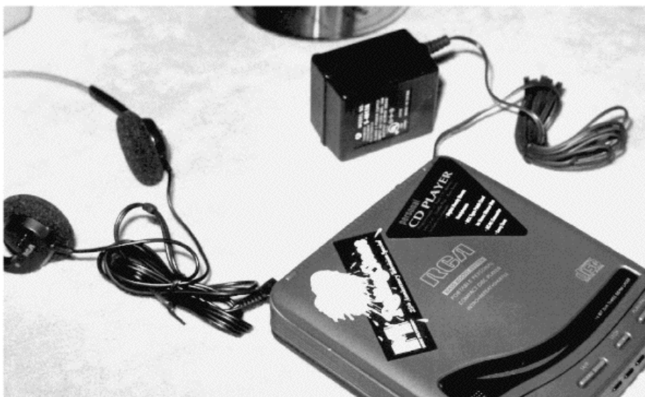
FIGURE 30-11 Plug in the small power supply when the CD portable is operated indoors.
