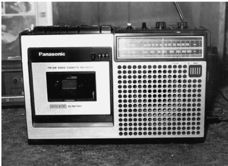
FIGURE 16-1 A large 5-inch pin-cushion speaker in the Panasonic RQ-542AS AM/FM radio cassette recorder.
