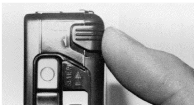
FIGURE 18-2 To pause momentarily, place the Pause switch in the direction of the arrow.
