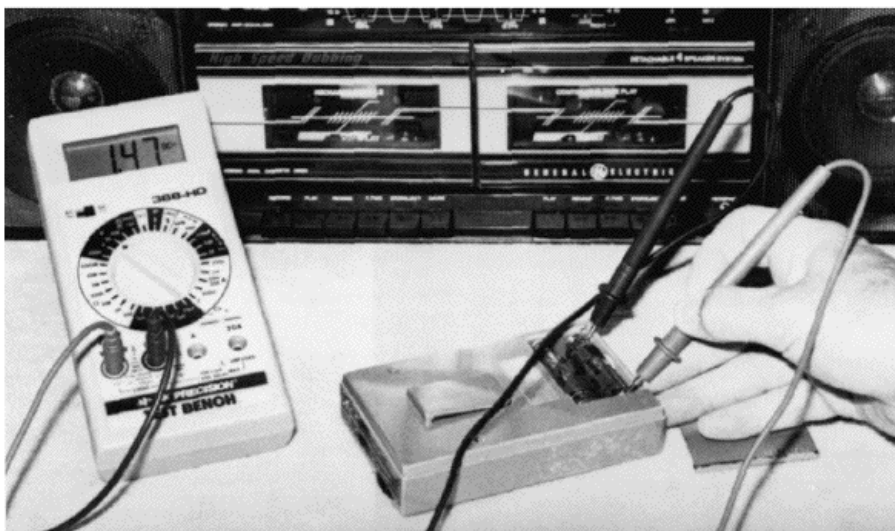
FIGURE 14-8 Check the batteries in the cassette player while it is operating to determine if they are weak and used up.
