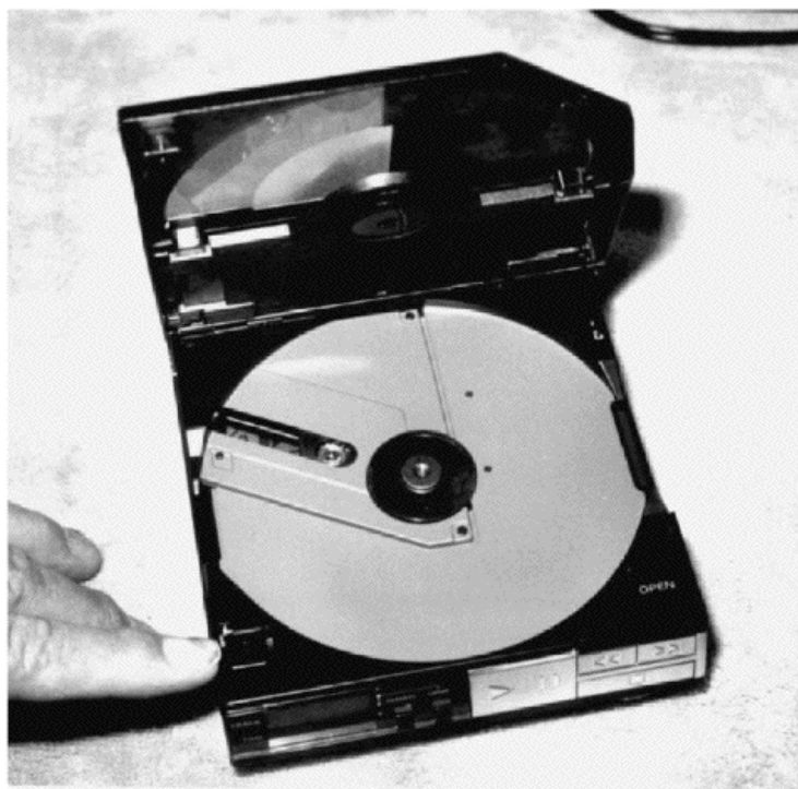
FIGURE 30-21 The lid switch shuts down the player when the lid or door is open.
