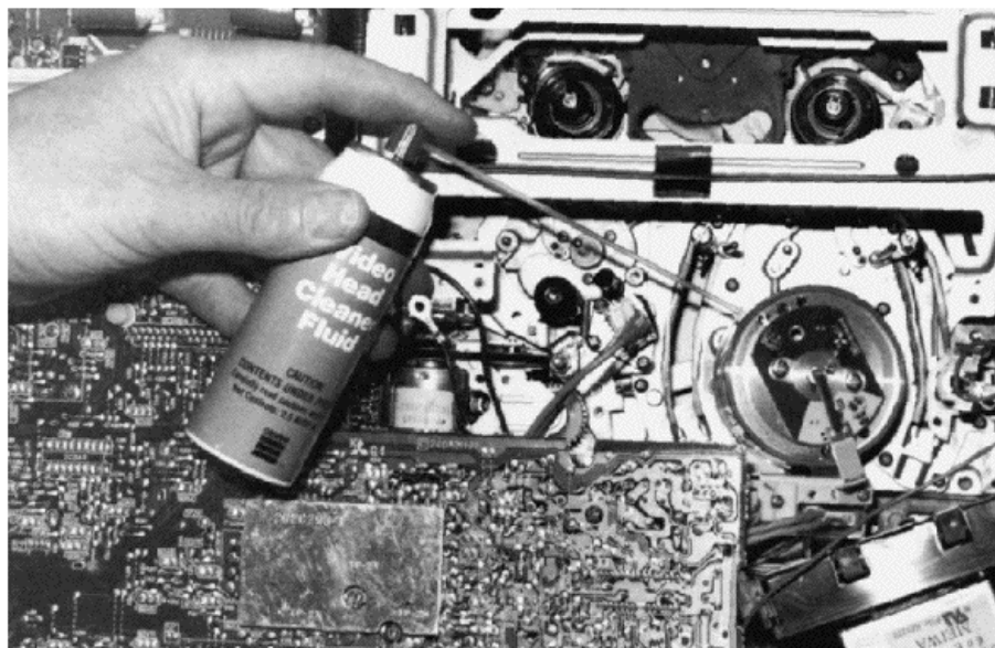
FIGURE 21-14 Head-cleaning spray can be used to clean dust from the various tape heads.
