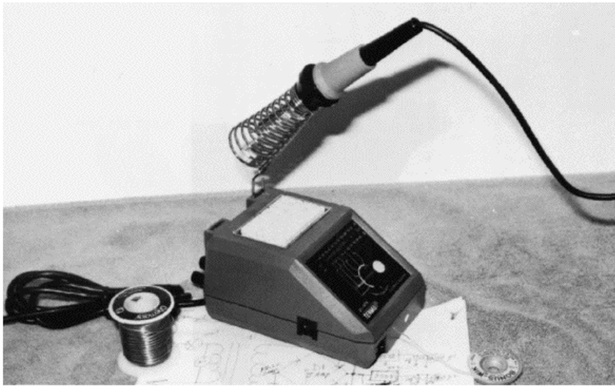
FIGURE 14-7 The temperature-controlled soldering iron is nice if you have a lot of soldering to do when servicing cassette players.
