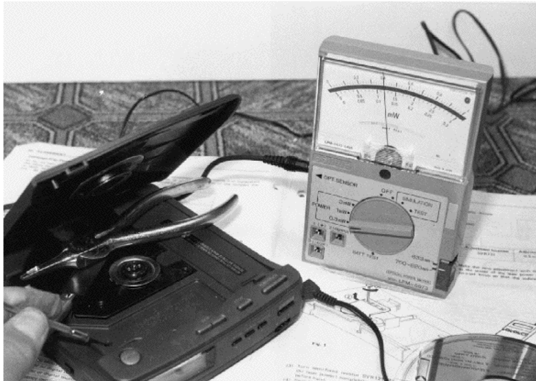
FIGURE 1-13 Besides the test instruments found upon the TV bench, the optical power meter, frequency counter, and AF signal generator are essential for compact disc (CD) servicing.
