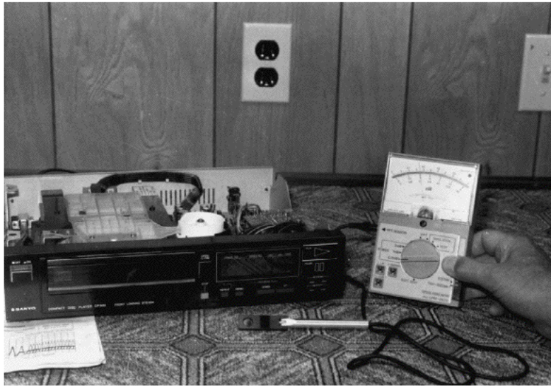
FIGURE 1-14 The optical power meter and special adjustment tools are necessary for CD servicing.
