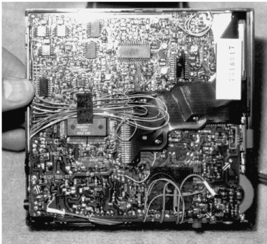
FIGURE 30-10 SMD components are on the bottom side of the PC board.
