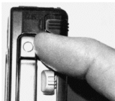
FIGURE 18-5 The Record switch is located on the right side of this Sony M-440 V-VOR Pressman microcassette recorder.
