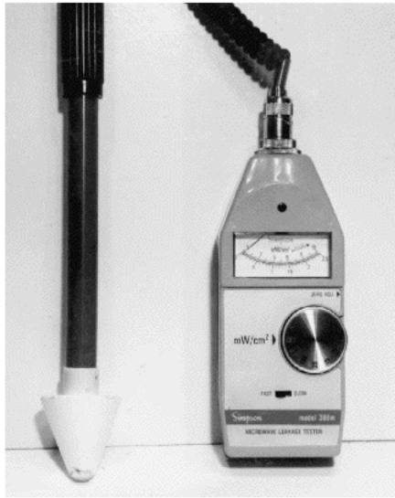
FIGURE 2-30 Check the oven for radiation with a U.S. government leakage standard survey meter.
