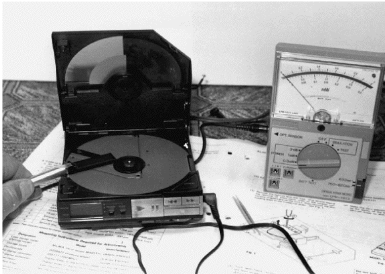
FIGURE 1-15 Besides checking the laser beam, the optical power meter can help you to check the LED, transmitting diode, and infrared remote-control units.
