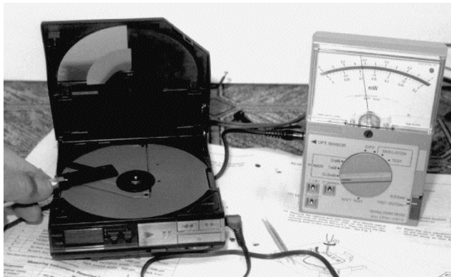
FIGURE 23-23 The laser power-meter probe is placed over the lens assembly to measure the power beam of the laser diode.
