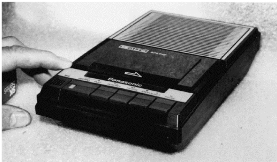
FIGURE 15-59 This Panasonic RQ-2103 cassette player operates from four C batteries.
