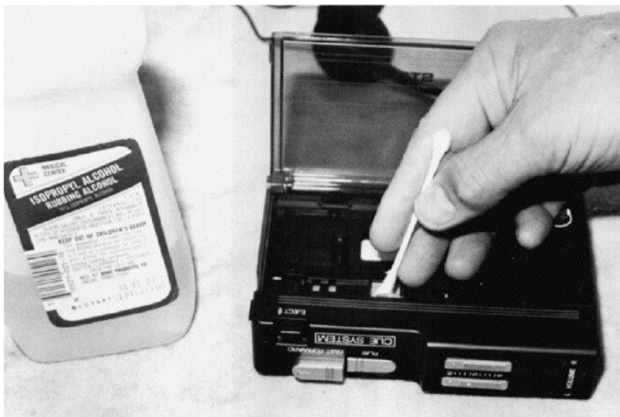
FIGURE 15-7 Clean the tape head with a high grade of isopropyl alcohol and a cleaning stick.
