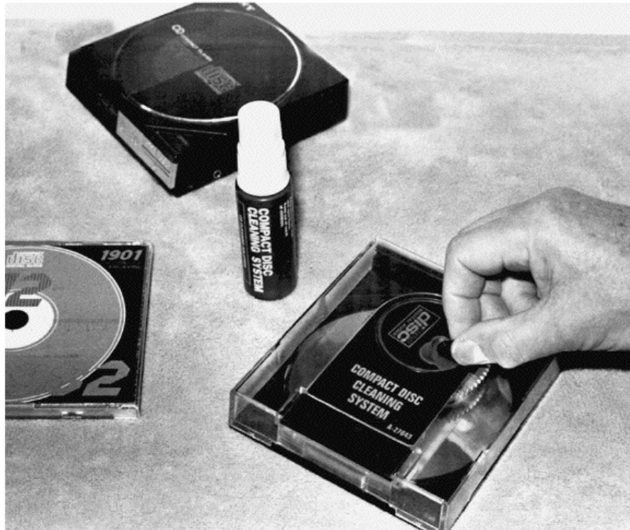
FIGURE 22-7 After cleaning and playing the disc, always place it back inside the plastic jewel box.
