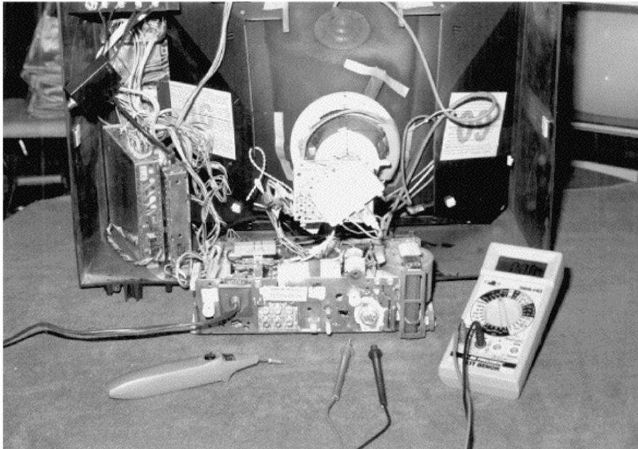
FIGURE 4-18 The horizontal output transistor is bolted to the metal chassis or heatsink in the RCA CTC108 chassis.
