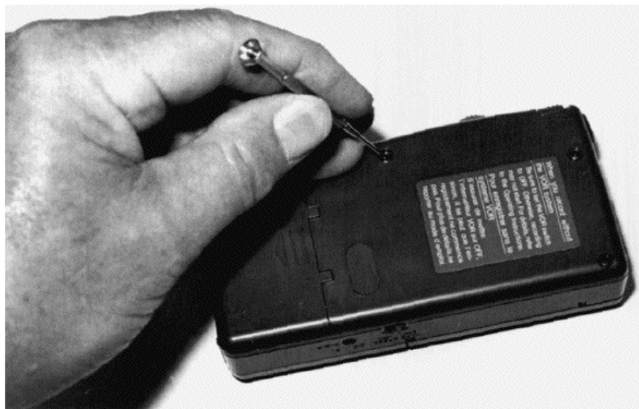
FIGURE 18-36 Remove four screws to remove the bottom panel of the Sony TCS-430 stereo cassette-recorder.
