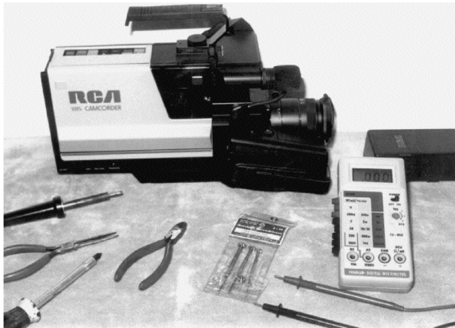
FIGURE 40-1 Choose small screwdrivers and tools to remove the various screws in the camcorder case.
