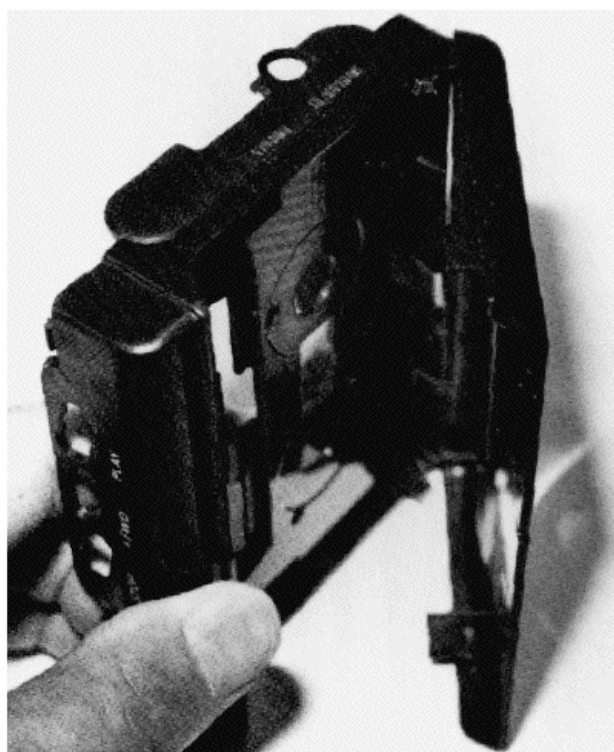
FIGURE 15-34 Replace the plastic cover or lid by snapping the small ends into the hub and spring area.
