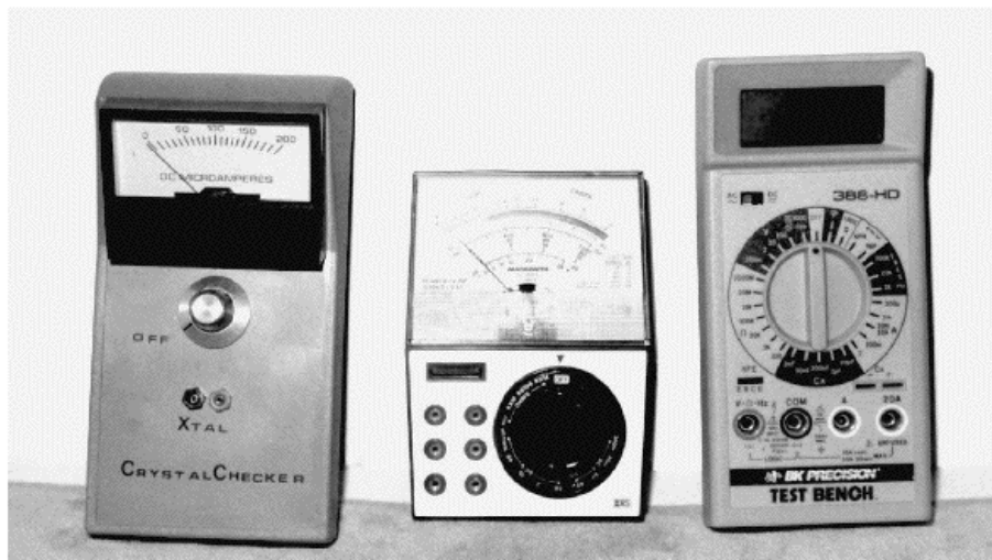
FIGURE 10-2 Besides the DMM, the crystal checker is another valuable test instrument for the color section.
