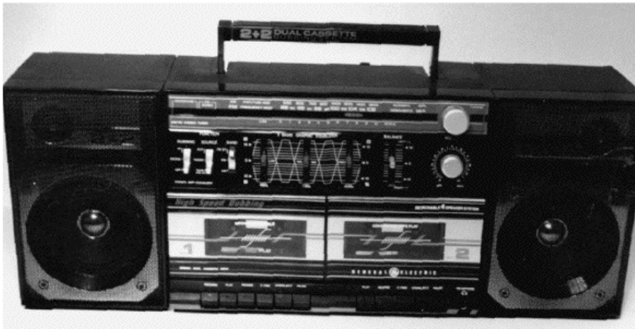
FIGURE 16-3 This GE boom box has dual cassette decks and an AM/FM-MPX stereo amplifier.
