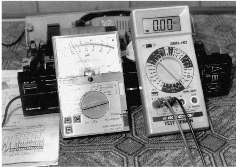
FIGURE 29-9 Checking remote-control transmitters with an infrared laser power meter.
