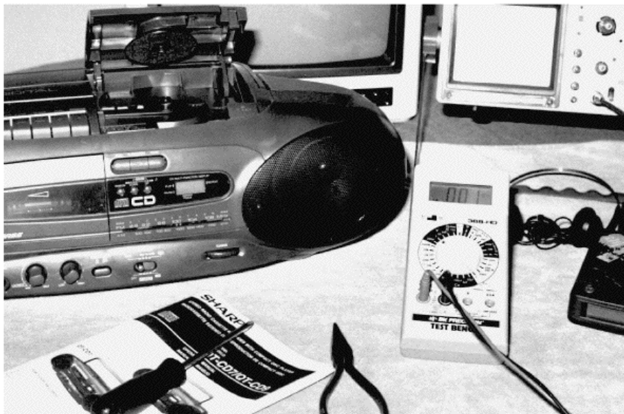
FIGURE 27-2 The CD player in this Sharp boom-box player uses the same audio amp and speakers.
