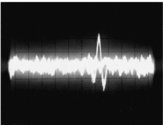
FIGURE 32-49 The focus error (FE) waveform.
