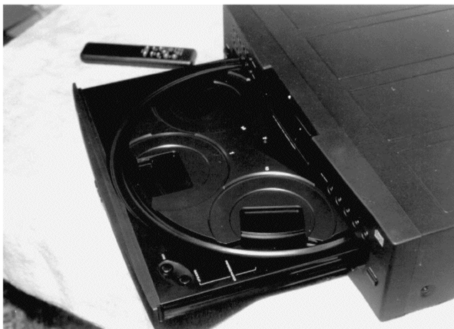
FIGURE 32-15 Check for binding rails if the loading is intermittent.
