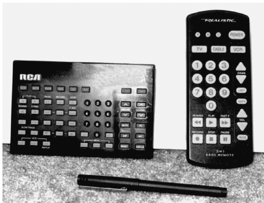
FIGURE 29-8 A universal remote control that operates TVs, VCRs, receivers, and CD players.
