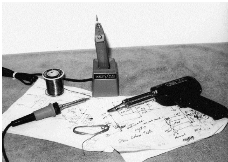
FIGURE 1-41 Use a soldering pencil or regulated soldering iron to replace SMD components.
