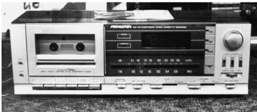
FIGURE 20-5 Most less-expensive decks use one motor for all functions, as in the Sounddesign deck.
