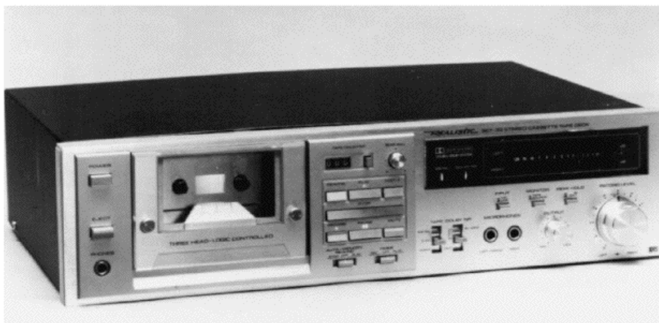
FIGURE 20-1 The cassette deck might include both Record and Play with stereo amplifiers or line-out connections.
