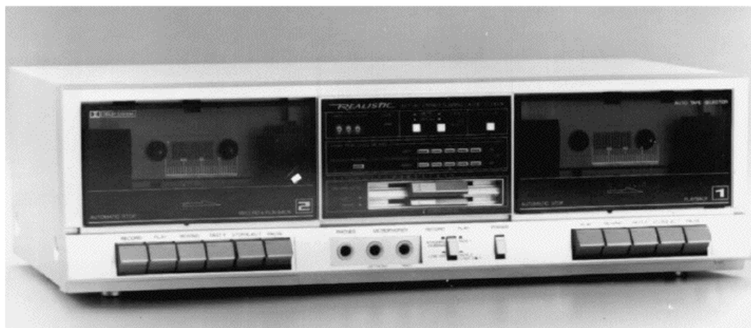
FIGURE 20-2 The cassette deck has dual decks; deck B records and plays and deck A only plays.
