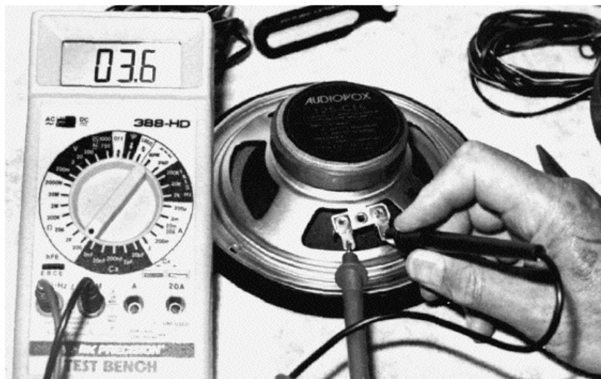
FIGURE 19-36 Check the voice-coil winding of a dead speaker with the R \times 1 range of an ohmmeter.
