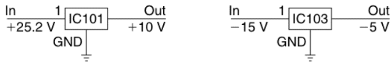
FIGURE 24-20 Check the output and input voltage sources on the IC or transistor regulators.
