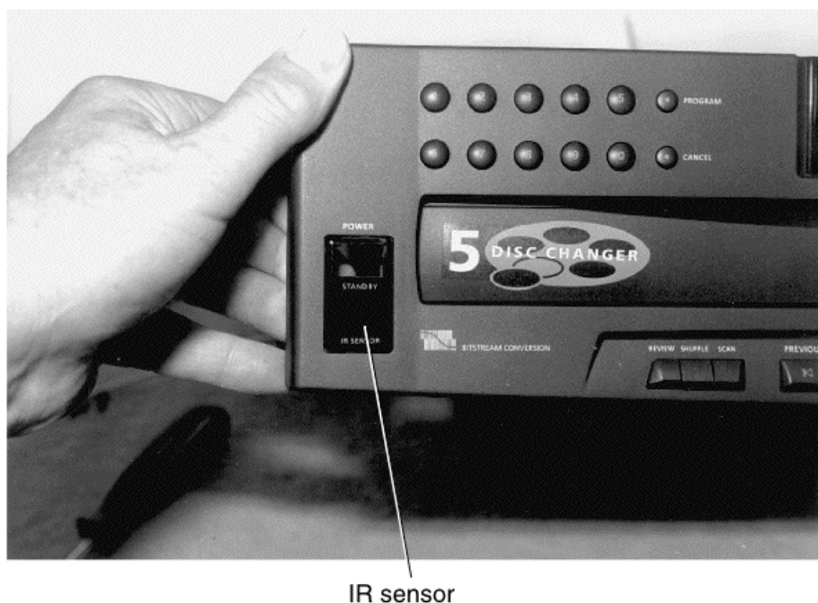
FIGURE 29-10 Here, the IR sensor is located on the front panel of a five-disc changer.
