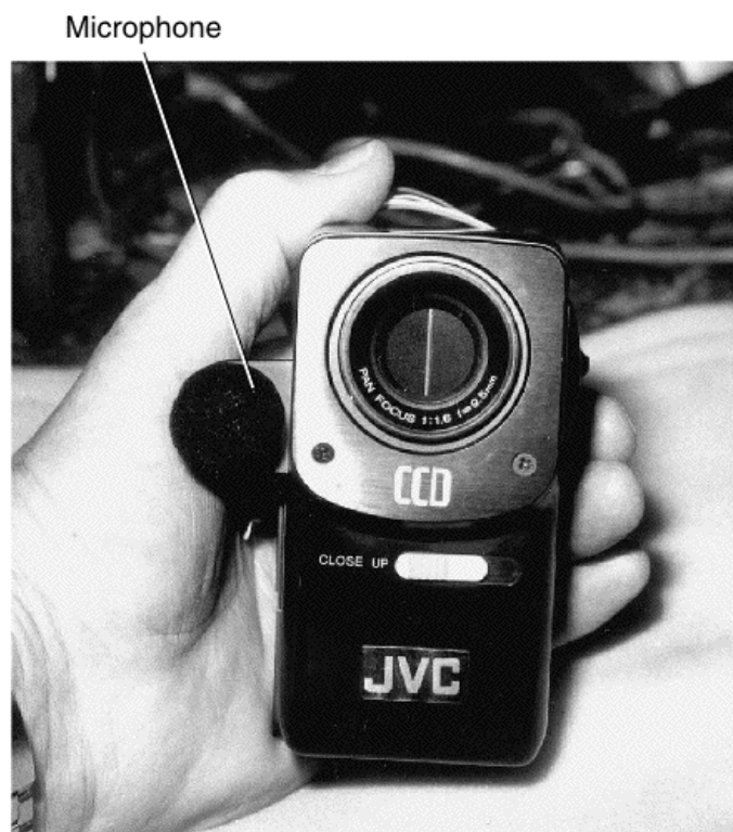
FIGURE 37-2 The condenser microphone is along side of the front of the camcorder.
