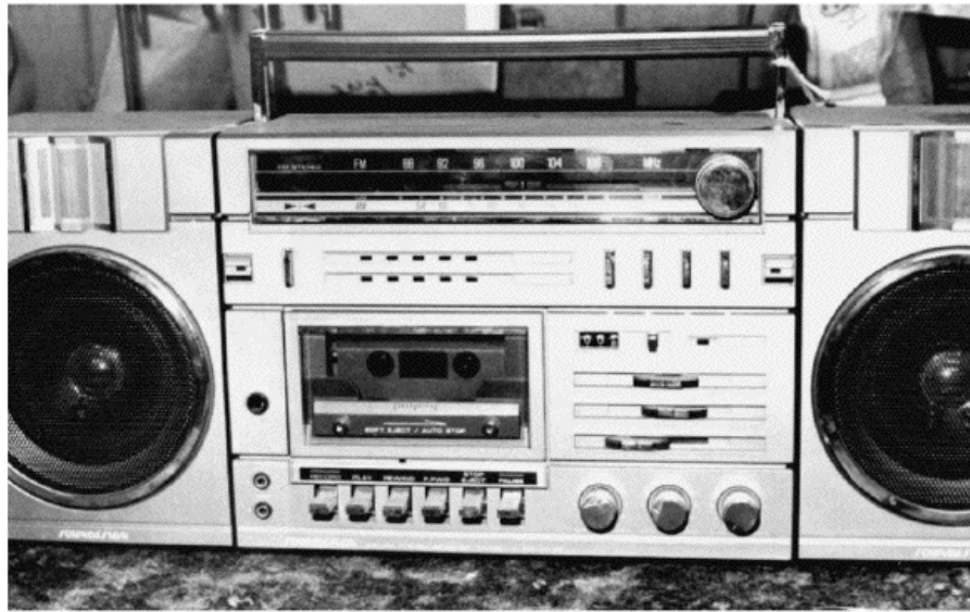
FIGURE 16-2 The large boom box might operate from 12 Vdc or from eight D cells.
