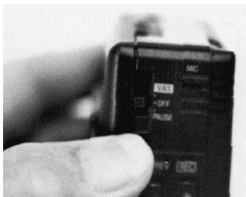
FIGURE 15-6 The VAS recording switch and level control in the Panasonic RQ-L315 recorder.
