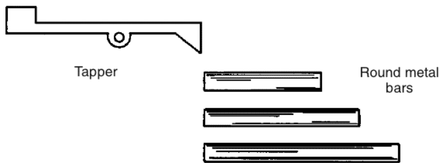
FIGURE 11-2 The mechanical plunger used in many early remote transmitters.
