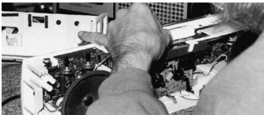
FIGURE 16-24 An electronic technician checking the recording circuits of a boom box.
