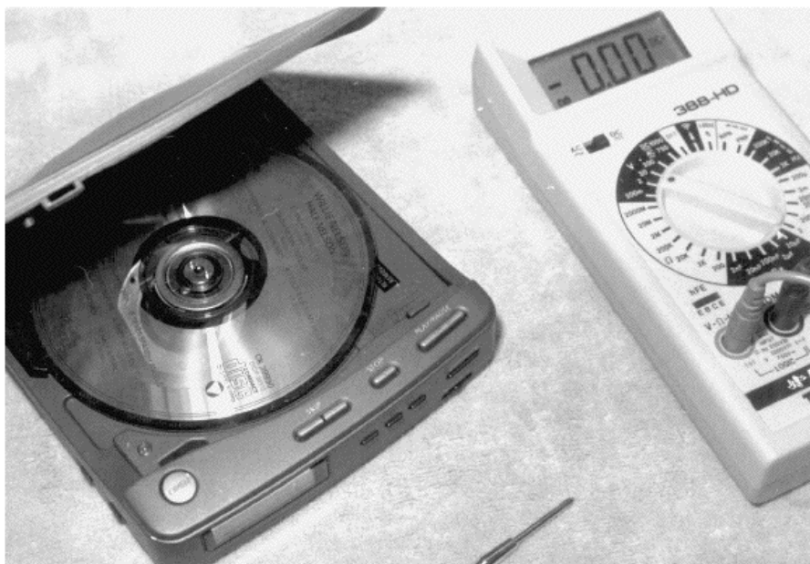
FIGURE 26-40 The CD disc lays on a small platform of disc motor in a portable CD player.
