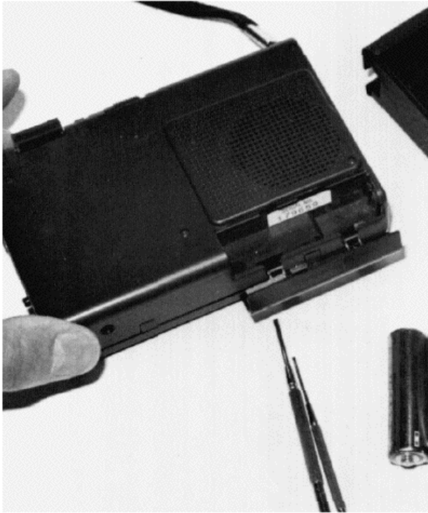
FIGURE 18-32 The small professional cassette player might operate from two AA batteries.
