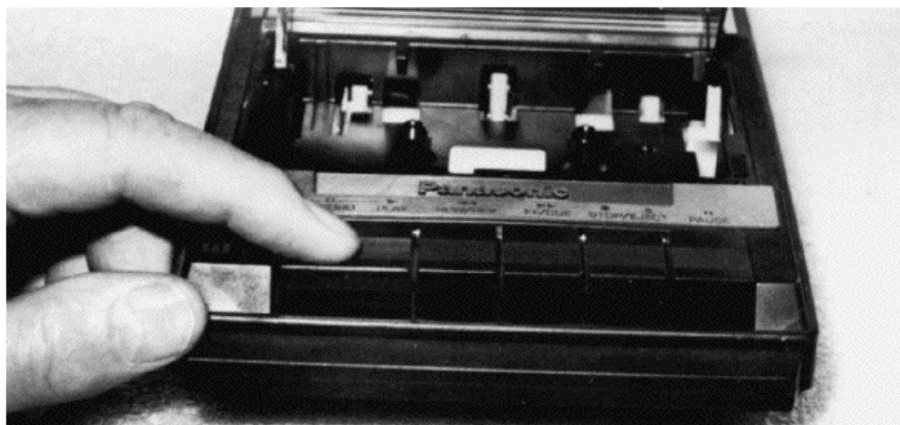
FIGURE 15-60 Cement broken plastic buttons with speaker or airplane glue.
