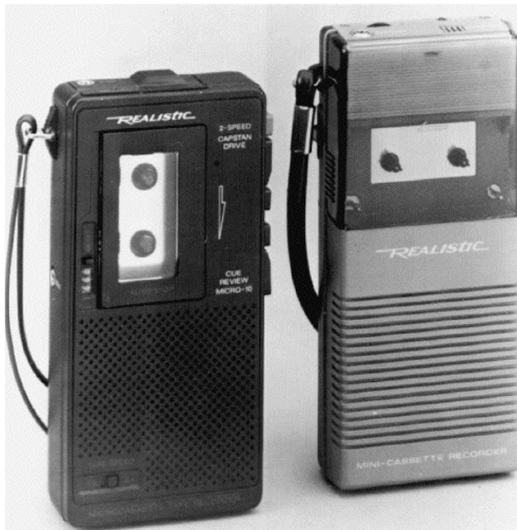
FIGURE 18-1 The small microcassette recorder might operate from two small AA batteries.
