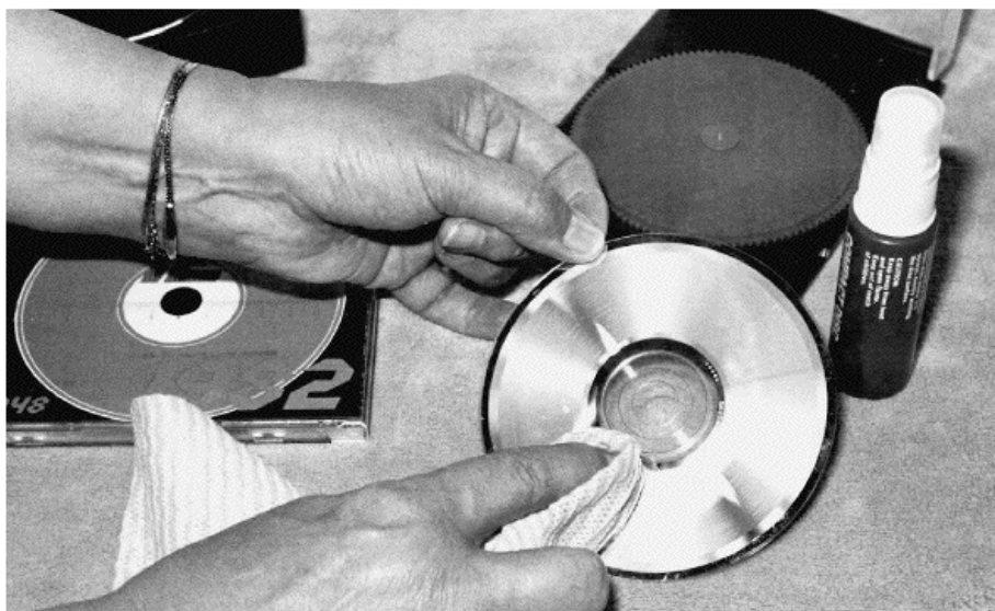
FIGURE 22-6 Clean the CD from the center toward the outside edge (radial-type cleaning).
