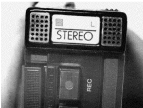
FIGURE 18-33 The TCS-430 professional cassette recorder has built-in twin stereo microphones.
