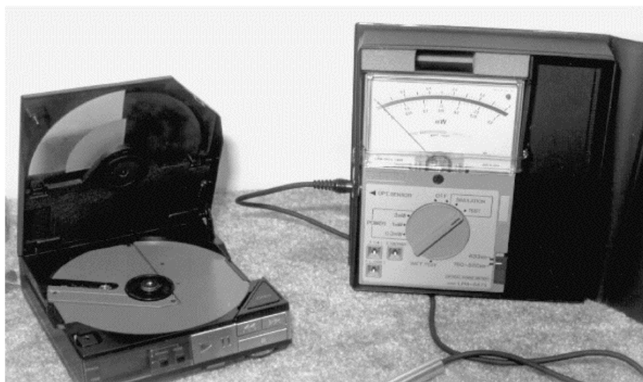
FIGURE 28-6 Check the laser diode with a portable laser power meter and check the manufacturer data.
