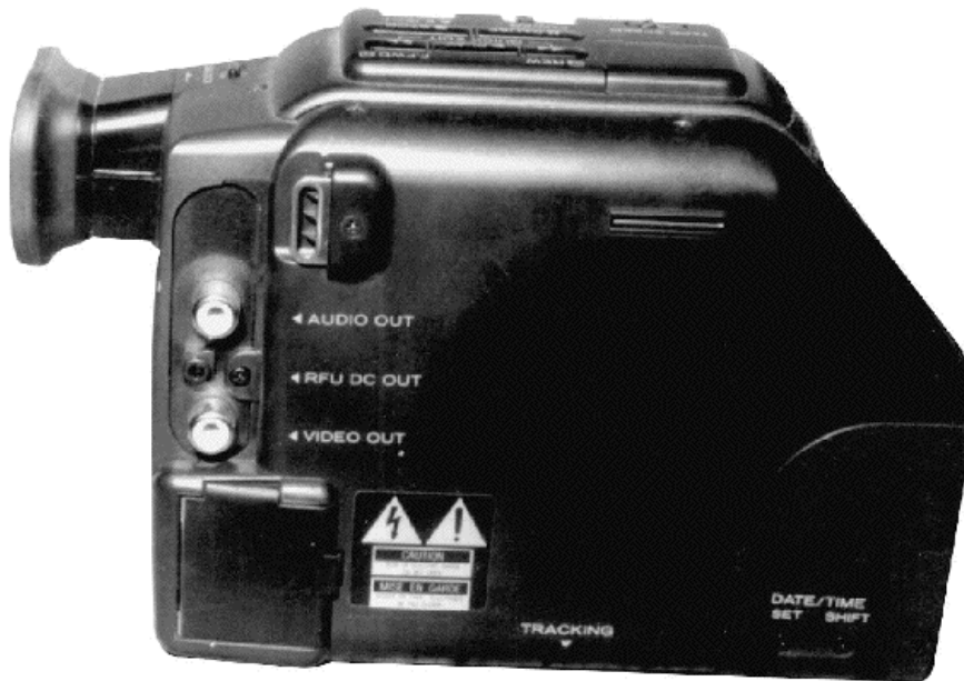
FIGURE 37-14 The audio and video output jacks are located at the back side of this Hitachi camcorder.
