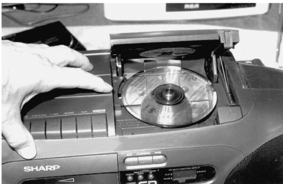
FIGURE 30-7 Top loading is also used in boom-box players.
