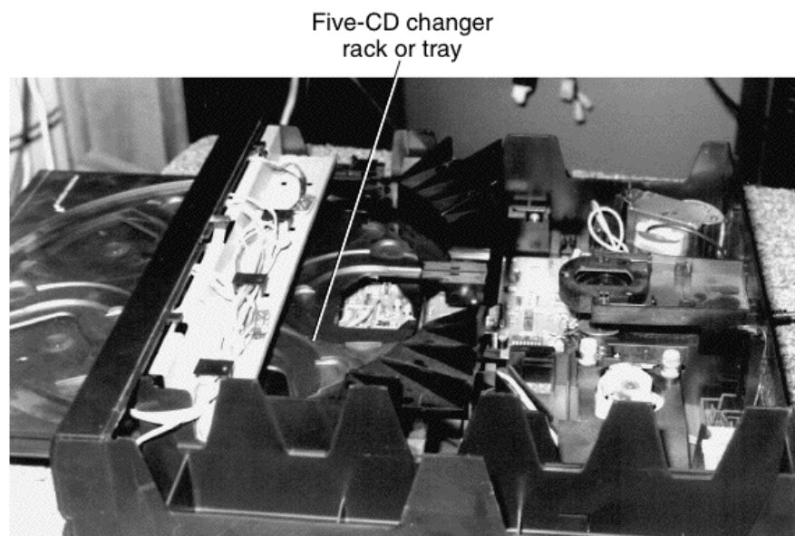
FIGURE 24-38 Displaced connecting wires caused the loading tray to hang up in this CDC-522 changer.
