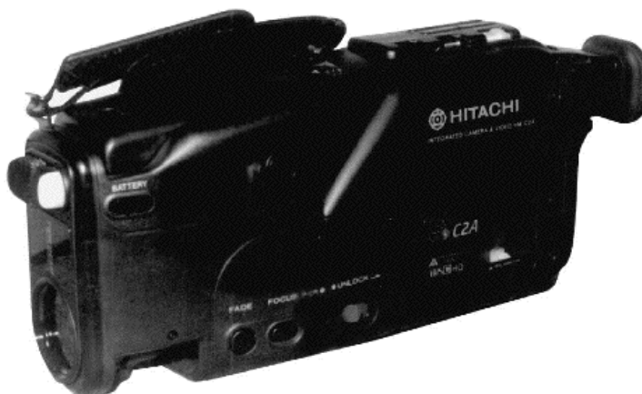
FIGURE 33-11 The electronic viewfinder is located at the rear of a Hitachi camcorder.
