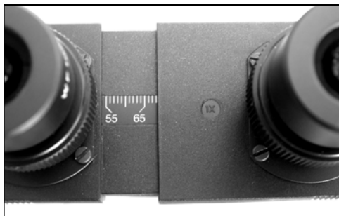
Fig. 3: Scale for adjusting the interpupillary distance.
