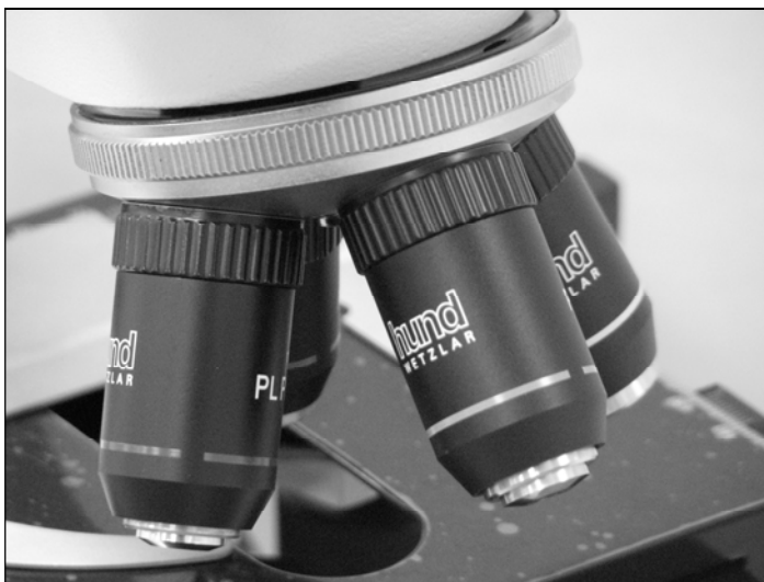
Fig. 29: Nosepiece for up to five objectives.
