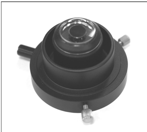
Fig. 44: Cardioid-type darkfield condenser NA 1.4.
