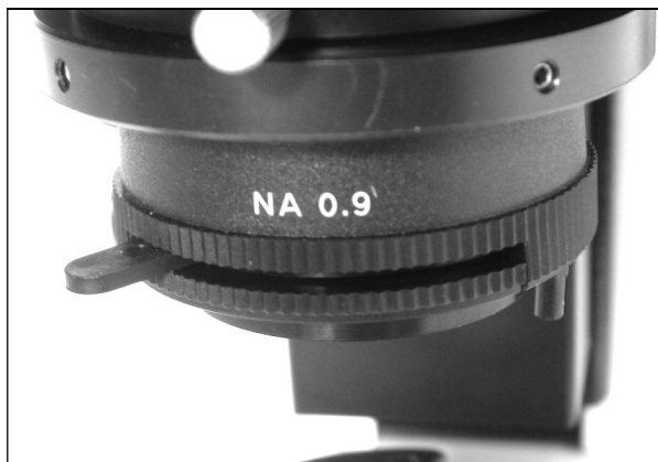
Fig. 40: Aperture diaphragm: adjustment lever.
