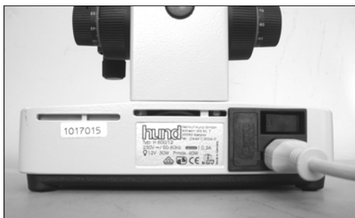
Fig. 8: Plugged mains cable.
