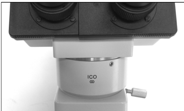
Fig. 30: Tube lens for infinity-corrected objectives.
