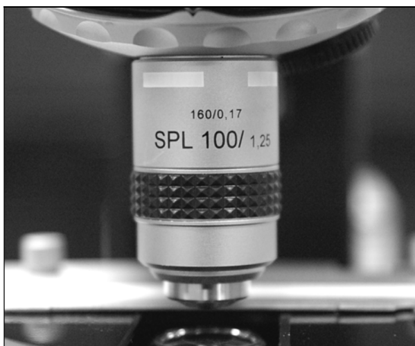
Fig. 45: Objective SPL 100/1.25 Oil with iris diaphragm.
