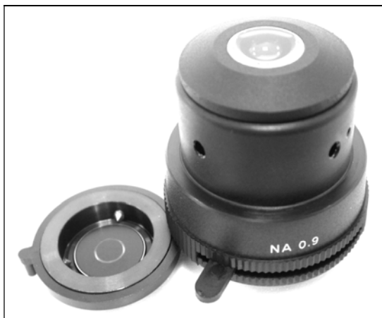
Fig. 22: Condenser NA 0.9 with annular diaphragm for phase contrast in filter holder.
