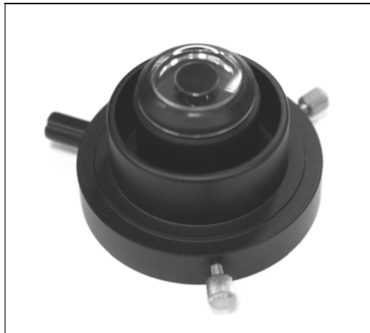
Fig. 25: Cardioid-type darkfield condenser NA 1.4.
