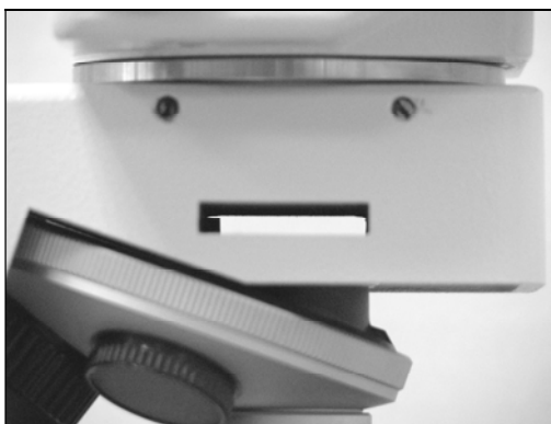
Fig. 31: Filter slit in microscope stand.
