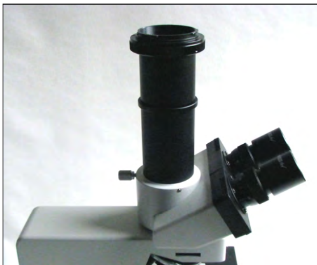
Fig. 36: Phototube with T2 adapter for single-lens reflex cameras.
