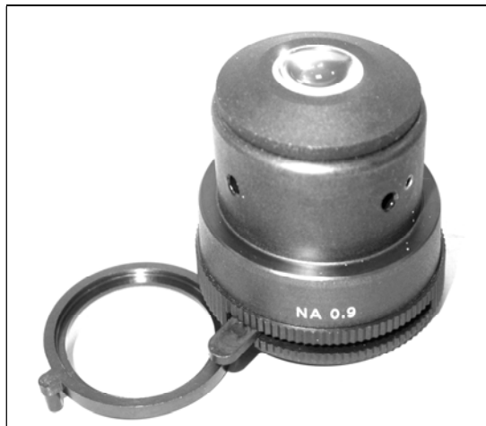
Fig. 21: Condenser NA 0.9 with filter holder and aperture diaphragm lever in fully opened position.
