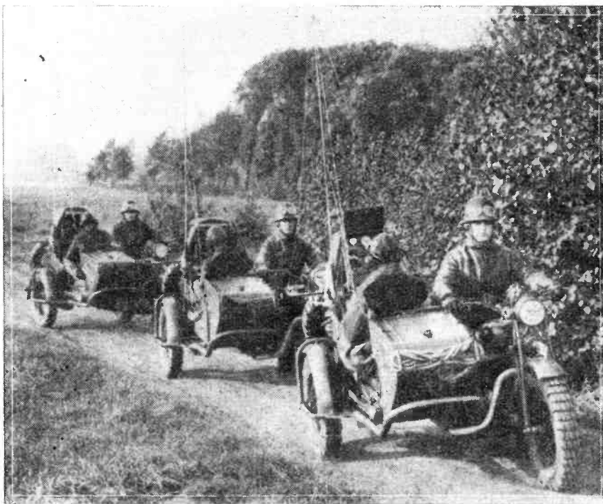
Motor-cycle combinations fitted with transmitting and receiving sets, being used during Belgian Army manoeuvres.
